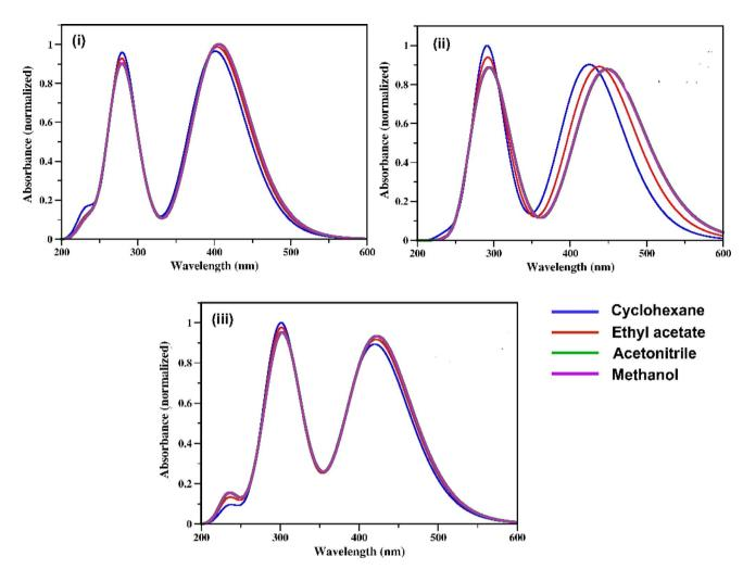
Fig. 3 Calculated electronic absorption spectra of the RFP chromophore analogue (i) 3a (ii) 3b and (iii) 3c in cyclohexane (blue,  $\varepsilon = 2.02$ ), ethyl acetate (red,  $\varepsilon = 6.02$ ) acetonitrile (green,  $\varepsilon = 35.688$ ), and methanol (violet,  $\varepsilon = 32.7$ ).
