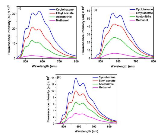
Fig. 2 Steady state fluorescence spectra of (i) 3a, (ii) 3b and (iii) 3c in cyclohexane, ethyl acetate, acetonitrile and methanol. Excitation wavelengths are 423 nm, 435 nm and 435 nm for 3a, 3b and 3c respectively. Concentration  $1 \times 10^{-5}$  M and bandpass 3, 3 nm are fixed for all fluorescence spectra.
