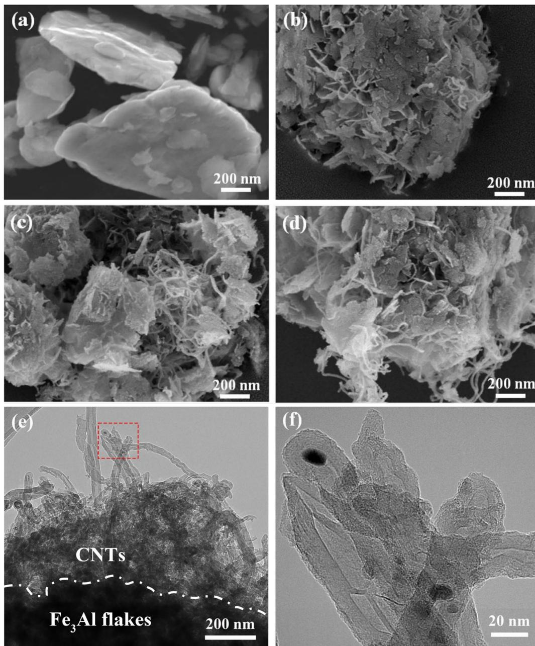
Fig. 1 Microstructure of  $\text{Fe}_3\text{Al}/\text{CNTs}$  composite absorbers obtained at different levels of CNT additions. (a)  $\text{Fe}_3\text{Al}$ , (b)  $\text{Fe}_3\text{Al}-0.5\%\text{CNT}$ , (c)  $\text{Fe}_3\text{Al}-1\%\text{CNT}$ , and (d)  $\text{Fe}_3\text{Al}-1.5\%\text{CNT}$ . (e) TEM image of  $\text{Fe}_3\text{Al}-1.5\%\text{CNT}$ . (f) Enlargement of (e) in the selective area (red square).
