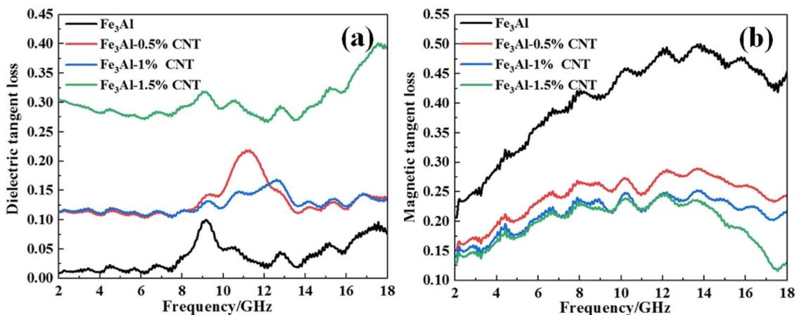
Fig. 5 Frequency dependence of (a) dielectric loss tangent and (b) magnetic loss tangent curves of the Fe<sub>3</sub>Al/CNTs composite absorbers.
