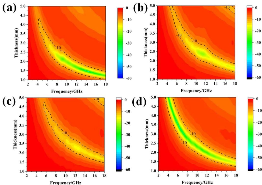
Fig. 7 Two-dimensional representation of the microwave reflection losses of  $\text{Fe}_3\text{Al}$ /CNT composite absorbers. (a)  $\text{Fe}_3\text{Al}$ , (b)  $\text{Fe}_3\text{Al}$ -0.5% CNT, (c)  $\text{Fe}_3\text{Al}$ -1% CNT, and (d)  $\text{Fe}_3\text{Al}$ -1.5% CNT.
