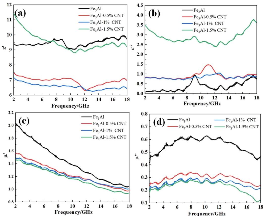
Fig. 4 Frequency dependence of (a) real and (b) imaginary parts of complex permittivity, frequency of dependence of (c) real and (d) imaginary parts of complex permeability curves of the Fe<sub>3</sub>Al/CNTs composite absorbers.
