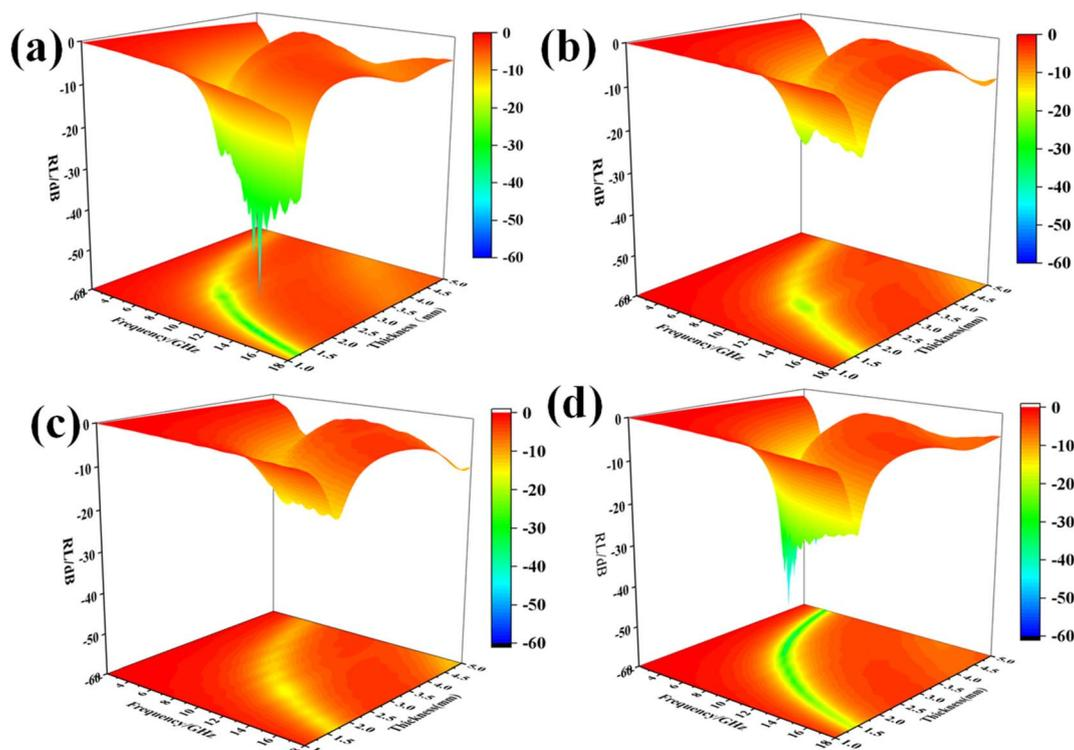
Fig. 6 Three-dimensional representation of the microwave reflection losses of the  $\text{Fe}_3\text{Al}/\text{CNT}$  composite absorbers. (a)  $\text{Fe}_3\text{Al}$ , (b)  $\text{Fe}_3\text{Al}-0.5\%$  CNT, (c)  $\text{Fe}_3\text{Al}-1\%$  CNT, and (d)  $\text{Fe}_3\text{Al}-1.5\%$  CNT.
