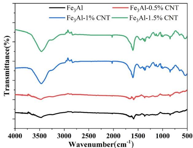
Fig. 3 FTIR spectra of the Fe<sub>3</sub>Al/CNTs composite absorbers.
