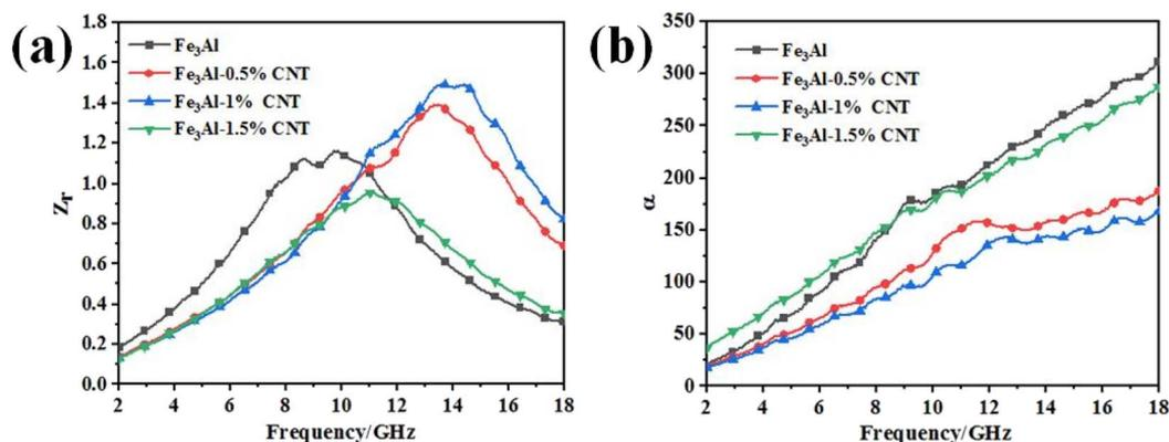
Fig. 9 (a) Impedance matching ratio and (b) attenuation constant  $\alpha$  of the Fe<sub>3</sub>Al/CNTs composite absorbers with a thickness of 2 mm.
