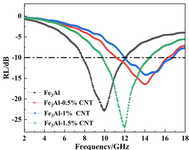
Fig. 8 Microwave reflection loss of the  $\text{Fe}_3\text{Al}$ /CNTs composite absorbers with a thickness of 2 mm.
