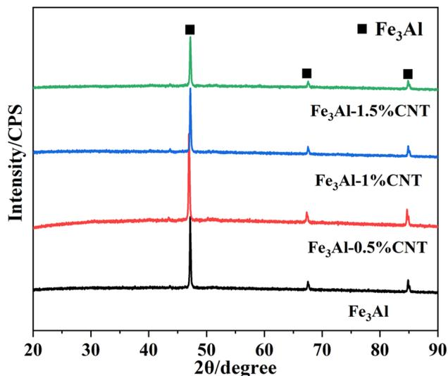
Fig. 2 XRD patterns of the Fe<sub>3</sub>Al/CNTs composite absorbers obtained with different CNT additions.
