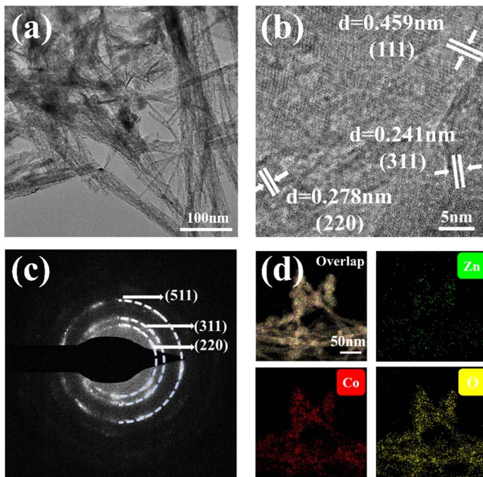
Fig. 2 (a) TEM image of  $\text{ZnCo}_2\text{O}_4\text{-}0.5$  nanoclusters. (b) HRTEM image, (c) SAED image, and (d) TEM elemental mapping analysis image of  $\text{ZnCo}_2\text{O}_4\text{-}0.5$  nanoclusters.
