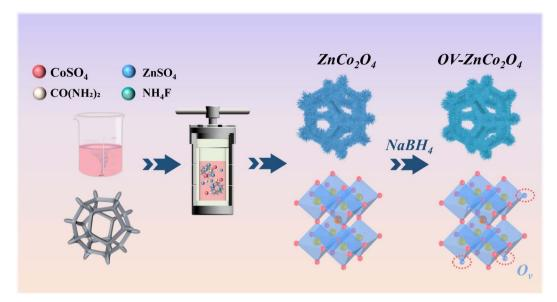
Scheme 1 The synthetic illustration of pristine ZnCo<sub>2</sub>O<sub>4</sub> and ZnCo<sub>2</sub>O<sub>4</sub>-0.5 nanoclusters.
