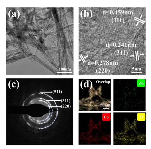
Fig. 2 (a) TEM image of  $ZnCo_2O_4$ -0.5 nanoclusters. (b) HRTEM image, (c) SAED image, and (d) TEM elemental mapping analysis image of  $ZnCo_2O_4$ -0.5 nanoclusters.
