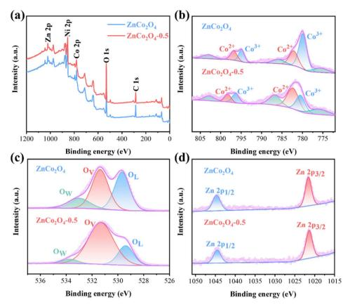
Fig. 3 XPS spectra of pristine ZnCo<sub>2</sub>O<sub>4</sub> and ZnCo<sub>2</sub>O<sub>4</sub>-0.5 nanoclusters: (a) wide-scan, (b) Co 2p, (c) O 1s and (d) Zn 2p.
