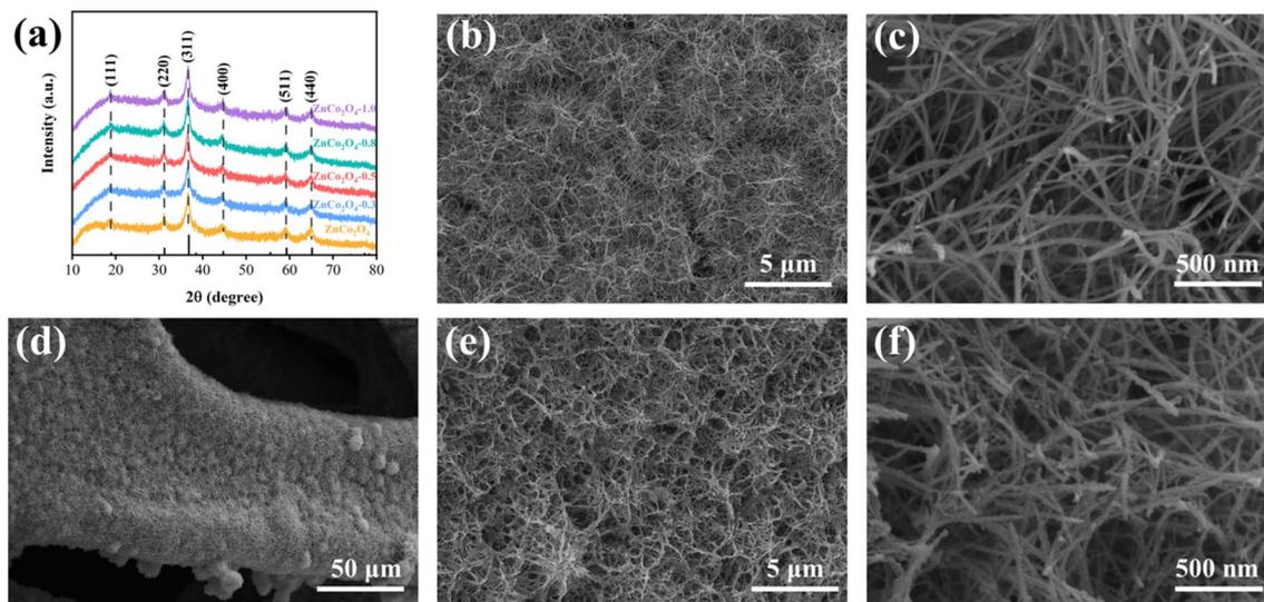
Fig. 1 (a) XRD patterns of  $\text{ZnCo}_2\text{O}_4$  and  $\text{OV-ZnCo}_2\text{O}_4$  (with different  $\text{NaBH}_4$  concentrations). (b and c) SEM images of pristine  $\text{ZnCo}_2\text{O}_4$  nanoclusters on NF. (d–f) SEM images of  $\text{ZnCo}_2\text{O}_4$ -0.5 nanoclusters on NF.
