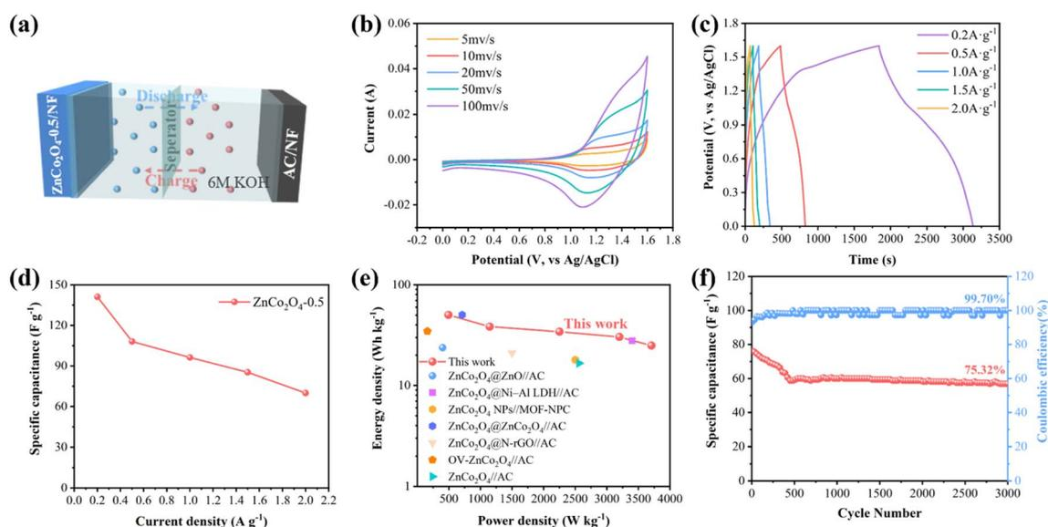
Fig. 5 Electrochemical performance of  $\text{ZnCo}_2\text{O}_4\text{-}0.5$  nanoclusters//AC ASC device. (a) Schematic pattern of as-assembled ASC device. (b) CV curves at different scan rates. (c) GCD curves at different current densities. (d) Specific capacitance at different current densities. (e) Ragone plots of energy and power densities. (f) Cycling performance and coulombic efficiency after 3000 cycles at  $2 \text{ A g}^{-1}$ .
