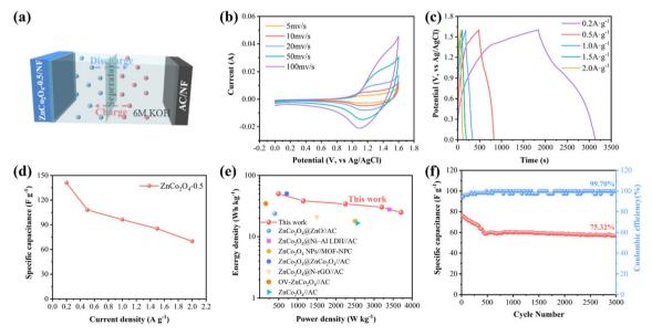
Fig. 5 Electrochemical performance of  $ZnCo_2O_4$ -0.5 nanoclusters//AC ASC device. (a) Schematic pattern of as-assembled ASC device. (b) CV curves at different scan rates. (c) GCD curves at different current densities. (d) Specific capacitance at different current densities. (e) Ragone plots of energy and power densities. (f) Cycling performance and coulombic efficiency after 3000 cycles at 2 A  $q^{-1}$ .
