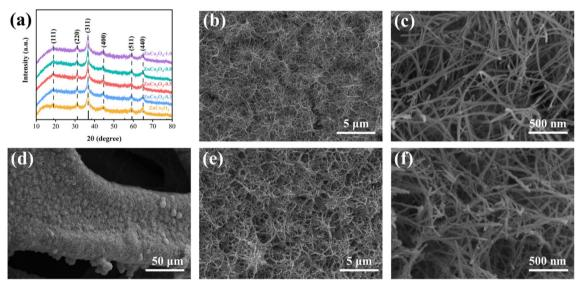
Fig. 1 (a) XRD patterns of  $ZnCo_2O_4$  and  $OV-ZnCo_2O_4$  (with different NaBH<sub>4</sub> concentrations). (b and c) SEM images of pristine  $ZnCo_2O_4$  nanoclusters on NF. (d-f) SEM images of  $ZnCo_2O_4-0.5$  nanoclusters on NF.
