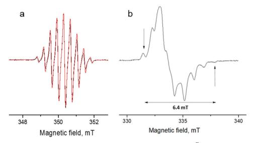
Fig. 8 Experimental (black) and simulated (red) continuous-wave (CW) X-band EPR spectra of DPP<sup>Th</sup>-NN<sub>2</sub> in toluene at room temperature (a) and in frozen toluene at 135 K (b) ( $C \approx 0.1$  mM).
