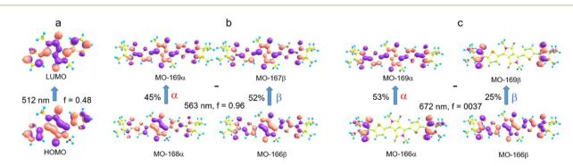
Fig. 6 Molecular orbitals (MO) involved in the long wavelength transition in the DPP<sup>Th</sup> spectrum (a), in the intense long wavelength transition in the DPP<sup>Th</sup>-NN<sub>2</sub> spectrum (b), and in the weak transition at 672 nm (c).
