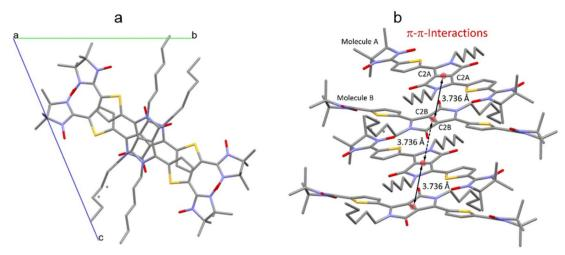
Fig. 3 (a) Solid state molecular packing of DPP<sup>Th</sup>-NN<sub>2</sub> with  $\pi-\pi$ -interactions; (b) side view of DPP<sup>Th</sup>-NN<sub>2</sub> with  $\pi-\pi$ -distances between centroids of the DPP<sup>Th</sup> moieties.
