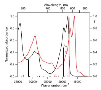
Fig. 5 Normalized electronic absorption spectra of the DPP<sup>Th</sup> precursor (black curve) and DPP<sup>Th</sup>-NN<sub>2</sub> diradical (red curve) measured in toluene at room temperature, as well as the calculated positions and oscillator strengths (*f*, right axis) of electronic transitions depicted as black bars for DPP<sup>Th</sup> and red bars for DPP<sup>Th</sup>-NN<sub>2</sub>.
