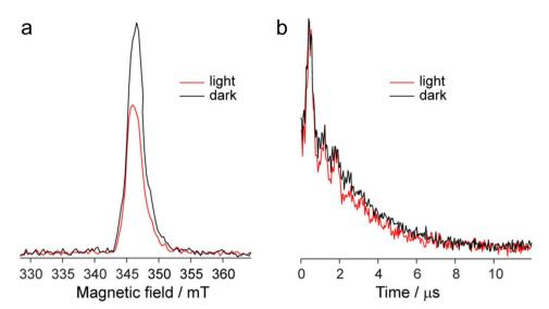
Fig. 9 Echo-detected EPR spectra (a) and phase relaxation kinetics (two-pulse echo decay vs. interpulse delay) (b) the DPP<sup>Th</sup>-NN<sub>2</sub> diradical in toluene glass at T=10 K in the presence/absence of photoexcitation. Kinetic curves are normalized to the maximum.
