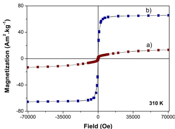
Fig. 12 310 K-isothermal variation of the magnetization as a function of the magnetic field of citrate coated (a)  $\beta$ - $\text{NaY}_{0.8}[\text{Yb}_{0.18}\text{Er}_{0.02}]\text{F}_4$ @ $\gamma$ - $\text{Fe}_2\text{O}_3$  and (b)  $\gamma$ - $\text{Fe}_2\text{O}_3$  particles.
