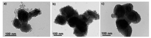
Fig. 4 TEM micrograph of an assembly of (a)  $\beta$ -NaY<sub>0.8</sub>[Er<sub>0.2</sub>]F<sub>4</sub>@ $\gamma$ -Fe<sub>2</sub>O<sub>3</sub>, (b)  $\beta$ -NaY<sub>0.8</sub>[Yb<sub>0.2</sub>]F<sub>4</sub>@ $\gamma$ -Fe<sub>2</sub>O<sub>3</sub> and (c)  $\beta$ -NaY<sub>0.8</sub>[Yb<sub>0.18</sub>Er<sub>0.02</sub>]F<sub>4</sub>@ $\gamma$ -Fe<sub>2</sub>O<sub>3</sub> particles.
