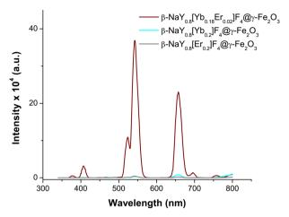
Fig. 6 Emission spectra of citrate coated β-NaY<sub>0.8</sub>[Yb<sub>0.18</sub>Er<sub>0.02</sub>]F<sub>4</sub>@γ-Fe<sub>2</sub>O<sub>3</sub> (wine line) β-NaY<sub>0.8</sub>[Yb<sub>0.2</sub>]F<sub>4</sub>@γ-Fe<sub>2</sub>O<sub>3</sub> (cyan line) and β-NaY<sub>0.8</sub>[Er<sub>0.2</sub>]F<sub>4</sub>@γ-Fe<sub>2</sub>O<sub>3</sub> (grey line) particles dispersed in Milli-Q water (1  $\mu$ g mL<sup>-1</sup>), recorded at r.t. after a laser irradiation of 980 nm.
