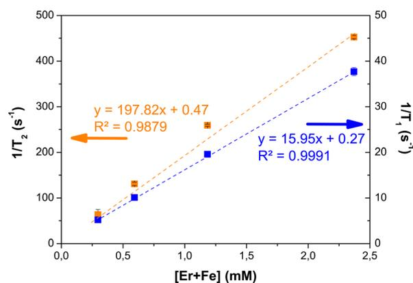
Fig. 13 Determination of the longitudinal ( $r_1$ ) and transverse ( $r_2$ ) relaxivities of citrate-coated  $\beta$ - $\text{NaY}_{0.8}[\text{Yb}_{0.18}\text{Er}_{0.02}]\text{F}_4$ @ $\gamma$ - $\text{Fe}_2\text{O}_3$  particles in Milli-Q water at 37 °C for an applied static field of 1.41 T, by plotting the relaxation rates (inverse of the relaxation times) for  $T_1$  (blue squares) and  $T_2$  (orange squares) versus the total paramagnetic cation concentration.
