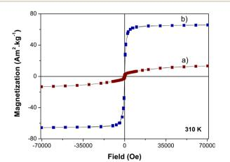
Fig. 12 310 K-isothermal variation of the magnetization as a function of the magnetic field of citrate coated (a)  $\beta$ -NaY<sub>0.8</sub>[Yb<sub>0.18</sub>Er<sub>0.02</sub>]F<sub>4</sub>@ $\gamma$ -Fe<sub>2</sub>O<sub>3</sub> and (b)  $\gamma$ -Fe<sub>2</sub>O<sub>3</sub> particles.
