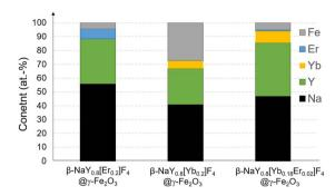
Fig. 1 XRF chemical analysis of the as-produced  $\beta$ -NaY<sub>0.8</sub>[Er<sub>0.2</sub>]F<sub>4</sub>@γ-Fe<sub>2</sub>O<sub>3</sub>,  $\beta$ -NaY<sub>0.8</sub>[Yb<sub>0.2</sub>]F<sub>4</sub>@γ-Fe<sub>2</sub>O<sub>3</sub> and  $\beta$ -NaY<sub>0.8</sub>[Yb<sub>0.18</sub>Er<sub>0.02</sub>]F<sub>4</sub>@γ-Fe<sub>2</sub>O<sub>3</sub> powders. Data accuracy (relative precision) was estimated to be less than 0.02 at% <sup>18</sup>
