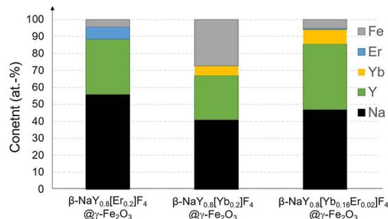
Fig. 1 XRF chemical analysis of the as-produced  $\beta$ -NaY<sub>0.8</sub>[Er<sub>0.2</sub>]F<sub>4</sub>@ $\gamma$ -Fe<sub>2</sub>O<sub>3</sub>,  $\beta$ -NaY<sub>0.8</sub>[Yb<sub>0.2</sub>]F<sub>4</sub>@ $\gamma$ -Fe<sub>2</sub>O<sub>3</sub> and  $\beta$ -NaY<sub>0.8</sub>[Yb<sub>0.18</sub>Er<sub>0.02</sub>]F<sub>4</sub>@ $\gamma$ -Fe<sub>2</sub>O<sub>3</sub> powders. Data accuracy (relative precision) was estimated to be less than 0.02 at%.<sup>18</sup>
