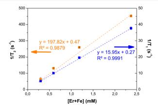
Fig. 13 Determination of the longitudinal  $(r_1)$  and transverse  $(r_2)$  relaxivities of citrate-coated β-NaY<sub>0.8</sub>|Yb<sub>0.18</sub>Er<sub>0.02</sub>|F<sub>4</sub>@γ-Fe<sub>2</sub>O<sub>3</sub> particles in Milli-Q water at 37 °C for an applied static field of 1.41 T, by plotting the relaxation rates (inverse of the relaxation times) for  $T_1$  (blue squares) and  $T_2$  (orange squares) *versus* the total paramagnetic cation concentration.
