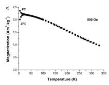
Fig. 11 Magnetization variation with temperature measured under the influence of a constant magnetic field of 500 Oe, following both field cooling (FC) and zero field cooling (ZFC) conditions for citrate coated (a) β-NaY<sub>0.8</sub>[Yb<sub>0.18</sub>Er<sub>0.02</sub>]F<sub>4</sub>, (b) γ-Fe<sub>2</sub>O<sub>3</sub> and (c) β-NaY<sub>0.8</sub>[Yb<sub>0.18</sub>Er<sub>0.02</sub>]F<sub>4</sub>@γ-Fe<sub>2</sub>O<sub>3</sub> particles.
