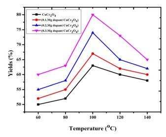
Fig. 6 Catalytic activity of the catalysts *versus* different reaction temperatures in the oxidation of veratryl alcohol. Reaction conditions: pure and doped samples: 0.3~g; alcohol: 10~mmol; acetonitrile: 10~mmol;  $H_2O_7$ : 10~mmol; time: 12~h; temperature: 60~to~140~°C.
