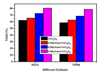
Fig. 9 Effect of oxidants in the selective oxidation of veratryl alcohol. Reaction conditions: pure and doped samples: 0.3 g; alcohol: 10 mmol; acetonitrile: 10 mmol; TBHP and  $H_2O_2$ : 10 mmol; time: 12 h; temperature: 100 °C.
