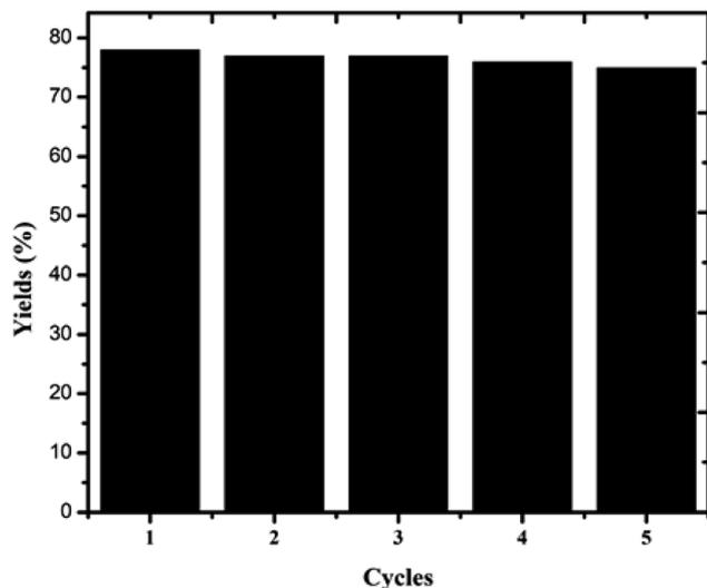
Fig. 10 Cycling performance of the copper chromite catalysts.
