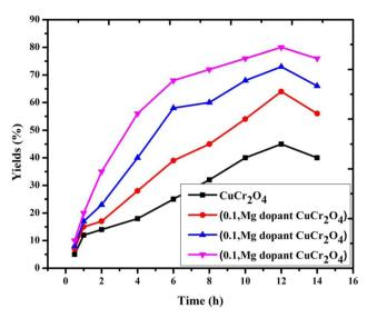
Fig. 8 Catalytic activity of the catalysts *versus* different reaction times for the selective oxidation of veratryl alcohol. Reaction conditions: pure and doped samples: 0.3 g; alcohol: 10 mmol; acetonitrile: 10 mmol;  $H_2O_2$ : 10 mmol; time: 0 to 16 h; temperature: 100 °C.
