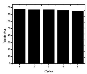
Fig. 10 Cycling performance of the copper chromite catalysts.
