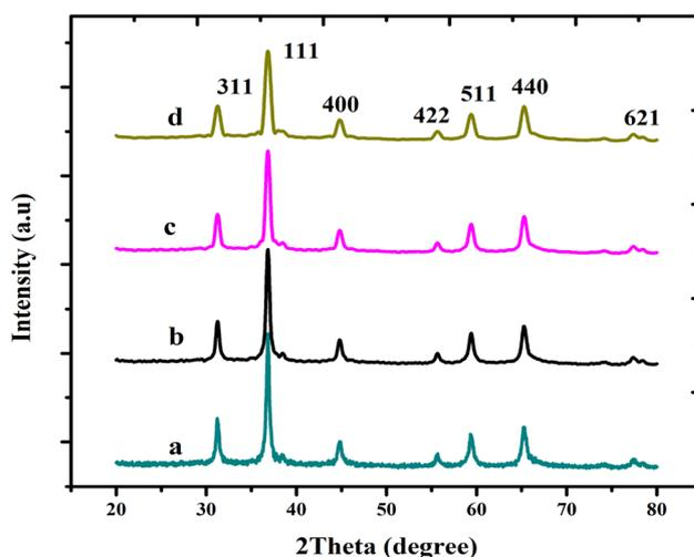
Fig. 1 X-ray diffraction pattern of (a) CuCr<sub>2</sub>O<sub>4</sub> and (b–d) Mg-doped CuCr<sub>2</sub>O<sub>4</sub>.
