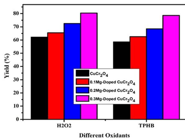
Fig. 9 Effect of oxidants in the selective oxidation of veratryl alcohol. Reaction conditions: pure and doped samples: 0.3 g; alcohol: 10 mmol; acetonitrile: 10 mmol; TBHP and  $\text{H}_2\text{O}_2$ : 10 mmol; time: 12 h; temperature: 100 °C.
