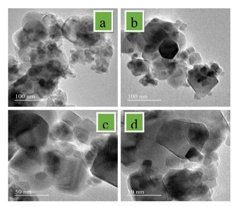
Fig. 4 TEM images of (a) CuCr<sub>2</sub>O<sub>4</sub> and (b-d) Mg-doped CuCr<sub>2</sub>O<sub>4</sub>.
