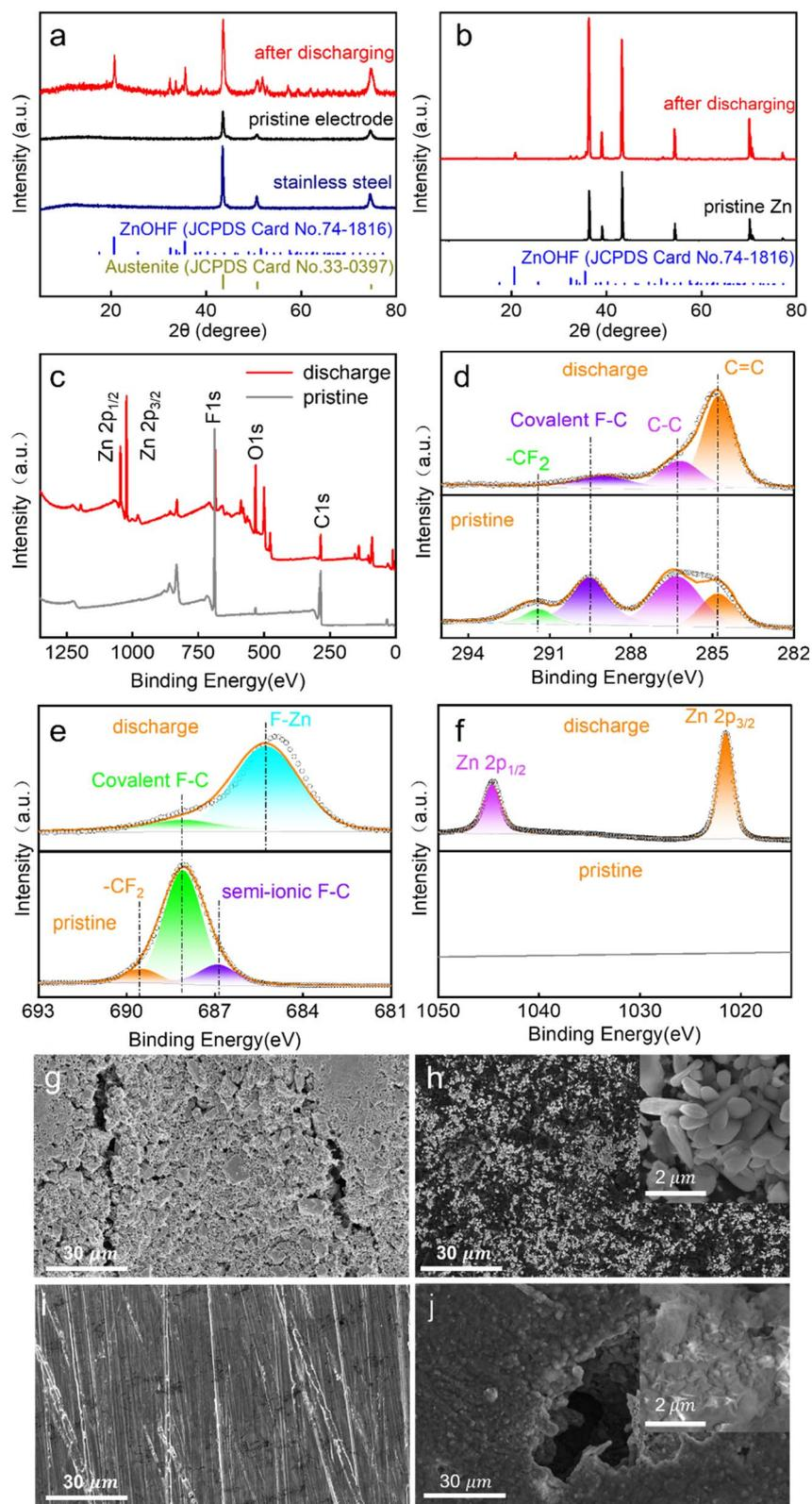
Fig. 4 XRD patterns of the (a)  $CF_{0.85}$  sample and (b) Zn discharge at  $30 \text{ mA g}^{-1}$ . XPS spectrum of (c) survey spectrum; (d) C 1s; (e) F 1s and (f) Zn 2p pristine and after discharge. SEM images of (g) pristine electrode, (h) electrode after discharge at  $30 \text{ mA g}^{-1}$ ; (i) pristine Zn after polishing; (j) Zn after discharging at  $30 \text{ mA g}^{-1}$ .
