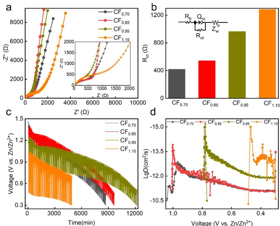
Fig. 3 (a) The impedance spectra, (b) fitted results of  $R_{ct}$  measured before discharge. Inset shows the equivalent circuit. (c) The discharge GITT curves of the four samples, (d) the calculated  $D$  from the GITT data for four samples as a function of potential during the discharge process.
