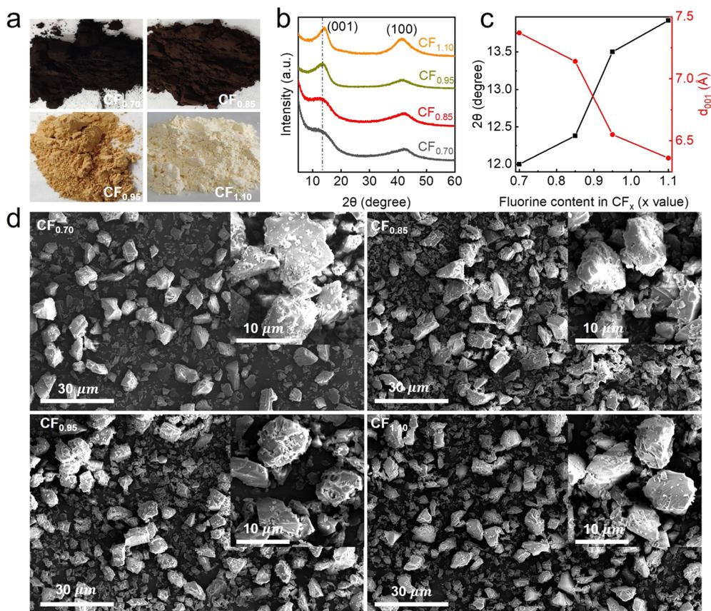
Fig. 1 (a) Images of the CF<sub>x</sub>. (b) XRD patterns of the CF<sub>x</sub>. (c) the degree and interlayer distance of the (001) diffraction peak. (d) SEM images of the samples.
