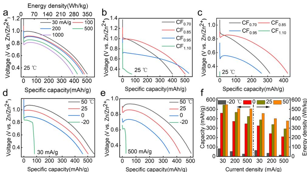
Fig. 2 (a) Galvanostatic discharge plots of the Zn/CF<sub>0.85</sub> cell at 25 °C, comparison of discharge curves of CF<sub>x</sub> at the 25 °C (b) 30 mA g<sup>-1</sup> and (c) 500 mA g<sup>-1</sup>. Comparison diagram of Zn/CF<sub>0.85</sub> battery at different temperatures (d) 30 mA g<sup>-1</sup>, (e) 500 mA g<sup>-1</sup>. (f) The corresponding capacity and energy density of the CF<sub>0.85</sub> sample.
