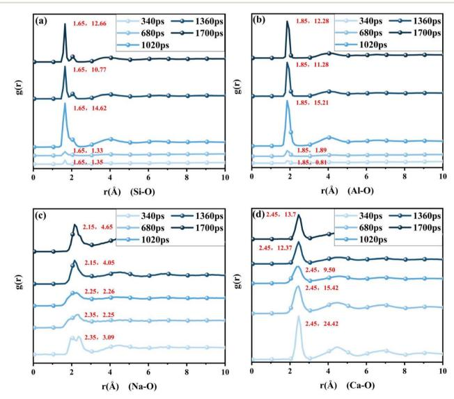
Plot of radial distribution function at different time stages (slag system): (a) Si-O; (b) Al-O; (c) Na-O; (d) Ca-O.
