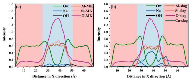
Fig. 4 (a) Atomic density distribution of metakaolin after activation; (b) atomic density distribution of slag after activation. Here, Na, OH, and Ow represent sodium ions, hydroxide ions, and oxygen atoms in water molecules of the NaOH solution respectively; Al-MK represents aluminum atoms in the metakaolin framework structure; the meanings of the other symbols are similar to the previous explanations.
