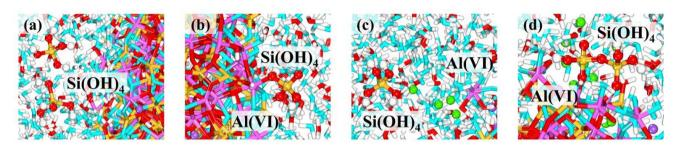
Fig. 6 (a) and (b) oligomers dissolved in MK system after alkali activation; (c) and (d) oligomers dissolved in slag system after alkali activation.
