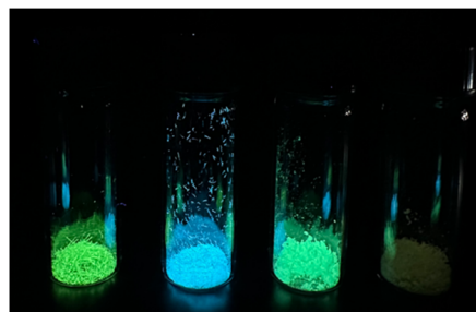
Fig. 2 Emission of p -anisil, BZL-OC9, BZL-OC12, and BZL-OC16 (left to right) under a hand-held UV lamp (365 nm).
