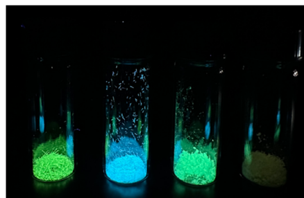
Fig. 2 Emission of p -anisil, BZL-OC9, BZL-OC12, and BZL-OC16 (left to right) under a hand-held UV lamp (365 nm).
