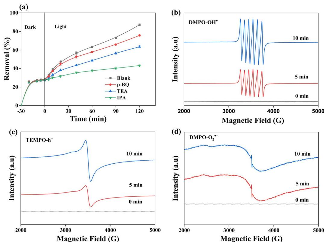
Fig. 7 (a) Effect of radicals' scavengers on the degradation performance of MNZ using PCN-600-NS-10. EPR spectra in different system: (b) DMPO-%  $\text{OH}^\bullet$ -adducts, (c) TEMPO-%  $\text{h}^+$  adducts, (d) DMPO-%  $\text{O}_2^{\bullet-}$  adducts (experimental conditions: catalysts =  $10 \text{ mg L}^{-1}$ , initial pH = 6, [DMPO] =  $20 \text{ mM}$ , [TEMPO] =  $20 \text{ mM}$ ).
