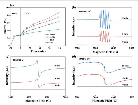
Fig. 7 (a) Effect of radicals' scavengers on the degradation performance of MNZ using PCN-600-NS-10. EPR spectra in different system: (b) DMPO- $^{\circ}$  OH $^{\circ}$ -adducts, (c) TEMP- $^{\circ}$  adducts, (d) DMPO- $^{\circ}$  %-adducts (experimental conditions: catalysts = 10 mg L $^{-1}$ , initial pH = 6, [DMPO] = 20 mM, [TEMP] = 20 mM).
