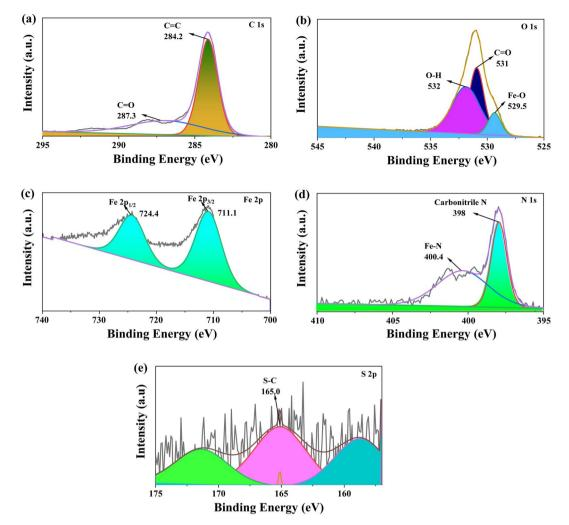
Fig. 3 XPS spectra of PCN-600-NS-10; (a) C 1s, (b) O 1s, (c) Fe 2p, (d) N 1s, and (e) S 2p.
