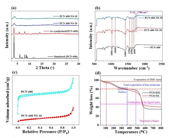
Fig. 1 XRD patterns (a) and FTIR spectra (b) of PCN-600, PCN-600-NS-10, and PCN-600-NS-20, (c) N<sub>2</sub>-adsorption desorption isotherms (c) and thermogravimetric analysis (d) of PCN-600 and PCN-600-NS-10
