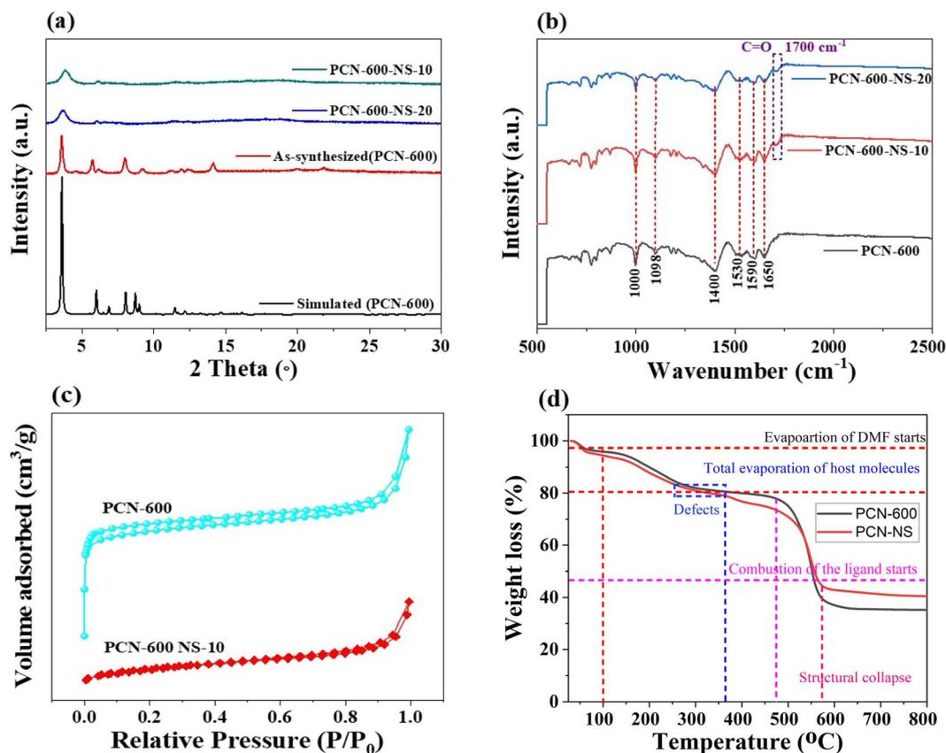
Fig. 1 XRD patterns (a) and FTIR spectra (b) of PCN-600, PCN-600-NS-10, and PCN-600-NS-20, (c) N<sub>2</sub>-adsorption-desorption isotherms (c) and thermogravimetric analysis (d) of PCN-600 and PCN-600-NS-10.
