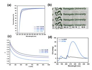
Fig. 7 (a) UV-vis transmittance spectra of P(nBA-co-AGluOH)s having different AGluOH contents (49-8 mol%) and (b) photographs of P(nBA-co-AGluOH)s films utilized for transmittance measurements, (c) wavelength-dependent refractive indices determined by ellipsometry, and (d) CD spectra of P(nBA-co-AGluOH) in HFIP (0.03 g L<sup>-1</sup>) and at the film state on a quartz plate
