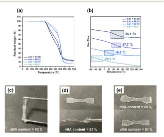
Fig. 3 (a) TGA traces (b) DSC traces of P(nBA-co-AGluOH)s (nBA content = 51-92 mol%) and (c-e) appearance of P(nBA-co-AGluOH) (nBA content = 51-92 mol%).
