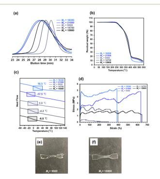
Fig. 6 (a) SEC, (b) TGA, and (c) DSC traces, and (d) stress-strain curves of P(nBA-co-AGluOH)s ( $M_n=9500-21500$ ) and (e and f) appearance of P(nBA-co-AGluOH)s ( $M_n=9500$ , 15 900).
