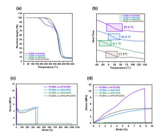
Fig. 4 (a) TGA traces (b) DSC traces of amino acid-based copolymers (nBA content = approximately 80 mol%) and (c and d) stress-strain curves of the random copolymers (nBA content = approximately 80 mol%) in (c) 0–1100% strain and (d) 0–10% strain.
