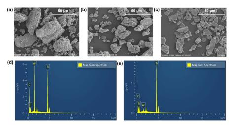
Fig. 2 SEM images of raw  $Ti_3AlC_2$  (a) and MXenes before (b) and after (c) DMSO treatment. EDS analysis of raw  $Ti_3AlC_2$  (d) and synthesized MXenes (e).
