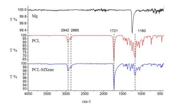
Fig. 4 FTIR spectra of Mg, PCL, and PCL-MXenes
