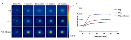
Fig. 6 Real-time infrared thermal images (A) and photothermal heating curves (B) of different samples immersed in NaCl under continuous 808 nm laser irradiation for 20 minutes.
