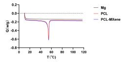
Fig. 7 DSC curves of Mg, PCL, and PCL-MXenes recorded in the  $10-120~^{\circ}$ C temperature range.
