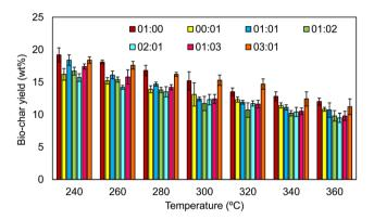
Fig. 6 Effect of temperature on biochar yield (%)
