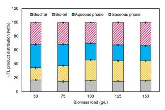
Fig. 7 Effect of biomass load
