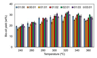
Fig. 5 Effect of temperature on bio-oil yield (%).
