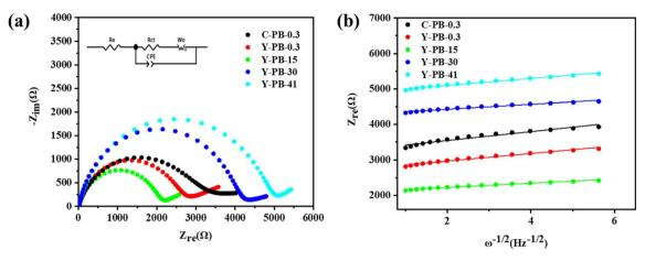
Fig. 6 (a) Nyquist plots of the impedance spectra for each sample (inset depicts the equivalent circuit model); (b) fitted curves of the real part of impedance ( $Z_{\rm re}$ ) as a function of  $\omega^{-1/2}$  in the low-frequency range.
