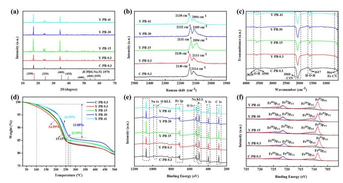
Fig. 2 XRD spectra (a), Raman spectra (b), FTIR spectra (c), TG curves (d), XPS spectra (e), Fe2p high-resolution spectra (f) of NaFeHCF samples.
