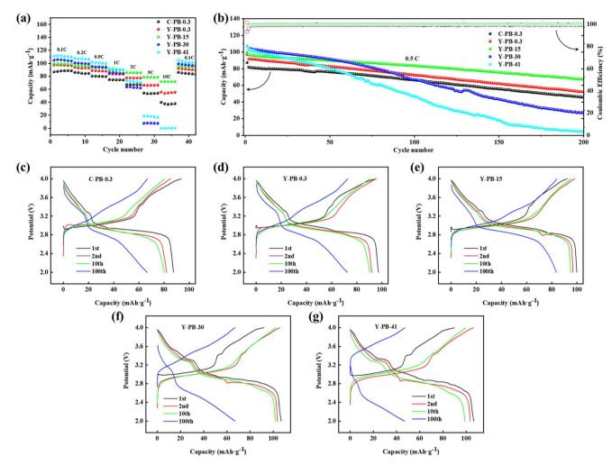
Fig. 4 Rate performance (a), cyclic performance at 0.5C (b) of each sample. Charge and discharge curves at 0.1C (first turn) and 0.5C (2nd, 10th, and 100th) for C-PB-0.3 (c), Y-PB-0.3 (d), Y-PB-15 (e), Y-PB-30 (f), and Y-PB-41 (g).
