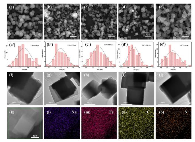
Fig. 3 SEM images of C-PB-0.3 (a), Y-PB-0.3 (b), Y-PB-15 (c), Y-PB-30 (d), and Y-PB-41 (e); particle size distribution graph of C-PB-0.3 (a'), Y-PB-0.3 (b'), Y-PB-15 (c'), Y-PB-30 (i), and Y-PB-41 (e'); TEM images of C-PB-0.3 (f), Y-PB-0.3 (g), Y-PB-15 (h), Y-PB-30 (i), and Y-PB-41 (j); EDS mapping results of Y-PB-15 (k-o).
