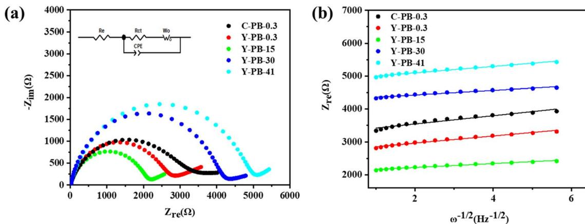
Fig. 6 (a) Nyquist plots of the impedance spectra for each sample (inset depicts the equivalent circuit model); (b) fitted curves of the real part of impedance ( $Z_{re}$ ) as a function of  $\omega^{-1/2}$  in the low-frequency range.
