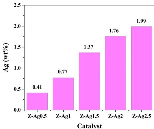
Fig. 1 Silver contents of Z-Ag0.5, Z-Ag1, Z-Ag1.5, Z-Ag2 and Z-Ag2.5 determined by ICP-OES.
