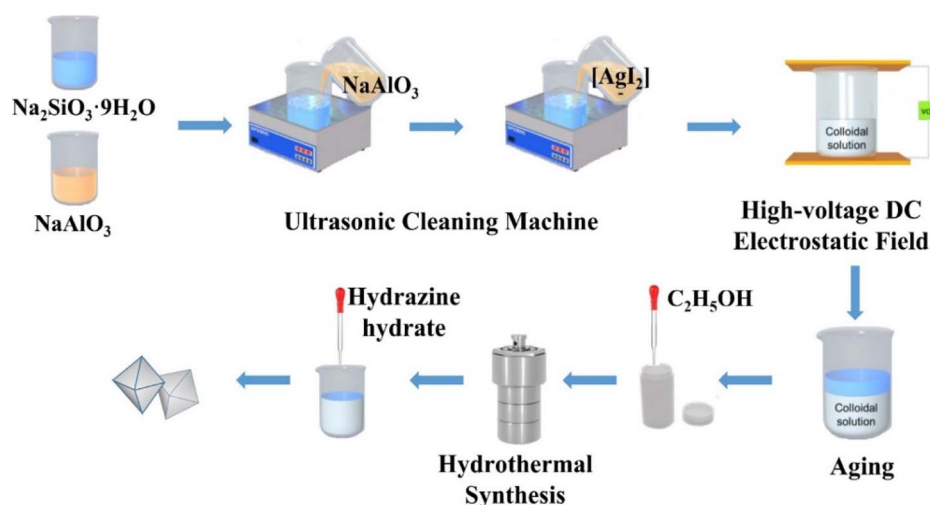
Scheme 1 The synthesis of octahedral 4 Å zeolite loaded Ag.
