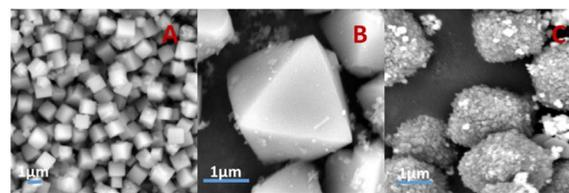
Fig. 6 SEM images of traditional 4 Å zeolites (A), and silver-loaded octahedral 4 Å zeolite before reduction (B) and after reduction (C).
