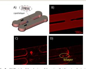
Fig. 3 (A) Sketch of the design of the microfluidic setup featuring a H-junction. (B–D) Fluorescence microscope images (lipids are stained with Rhod-PE) monitoring the process of lipid bilayer formation from (B) initial flooding of the device with lipid-squalene solution, (C) slow injection of the buffer phase and (D) contacting the oil–buffer interfaces coated now with a lipid monolayer forming a bilayer at the contact.
