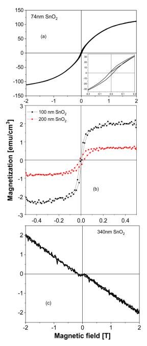
Fig. 3 Magnetization *versus* magnetic field taken at 300 K with field applied parallel to the film plane for  $SnO_2$  films with thickness as of (a) 74 nm; (b) 100 and 200 nm; and (c) 370 nm. The inset of (a) shows a zoom for M(H) of the 74 nm-thick film.
