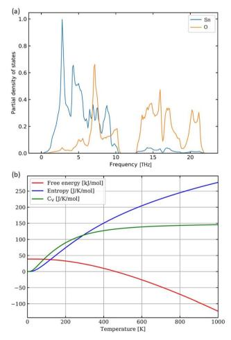
Fig. 6 Computed partial phonon densities of states of O and Sn within the SnO<sub>2</sub> rutile-structure bulk (a) and the corresponding temperature dependencies of thermodynamic quantities (b).
