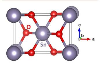
Fig. 5 A schematic visualization of the computational unit cell of the  $SnO_2$  with the rutile structure. Please note that some atoms are shown with their periodic images.
