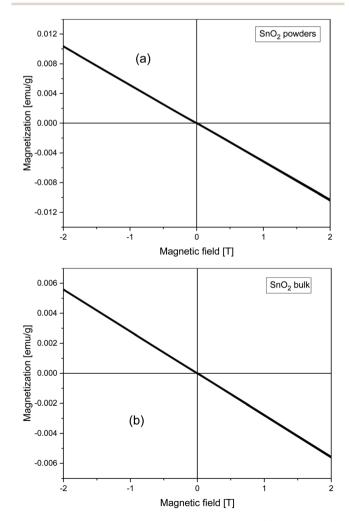
Fig. 2 Field dependence of magnetization taken at 300 K for the  $SnO_2$  (a) nano-powders and (b) bulk sample.
