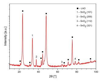
Fig. 1  $\,$  XRD pattern of a 74 nm-thick  $\rm SnO_2$  film deposited on  $\rm LaAlO_3$  substrate.
