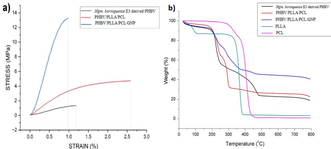
Fig. 4 (a) Stress vs. strain curve of PHBV derived from *Halogeometricum borinquense* E3 and its blend/composite. (b) Thermogravimetric curve of the haloarchaeal PHBV and its blend/composite<sup>45</sup> from 25 °C to 800 °C.
