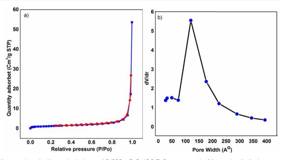
Fig. 7 (a) Nitrogen adsorption/desorption isotherm of CdSQDs@ZnCr-LDO/ZnO nanocomposite (b) pore size distribution according to BJH analysis.
