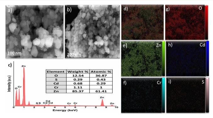
Fig. 4 Scanning electron microscopic images of (a) CdSQDs@ZnCr-LDO/ZnO nanocomposite and (b) EDX mapping for CdSQDs@ZnCr-LDO/ ZnO nanocomposite (c and d) elemental overlay for CdSQDs@ZnCr-LDO/ZnO nanocomposite and (e-i) the spectral mapping of each element in CdSQDs@ZnCr-LDO/ZnO
