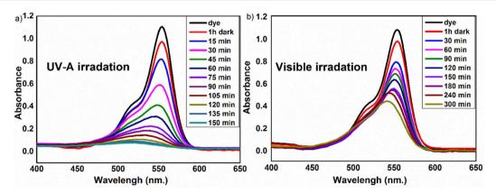
Fig. 9 Time-dependent progress of RhB photodegradation using the CdSQDs@ZnCr-LDO/ZnO ternary nanocomposites under (a) UV-A irradiation, and (b) fluorescent white light; ([catalyst] = 0.10 g L $^{-1}$ , initial RhB concentration [RhB] $_{
