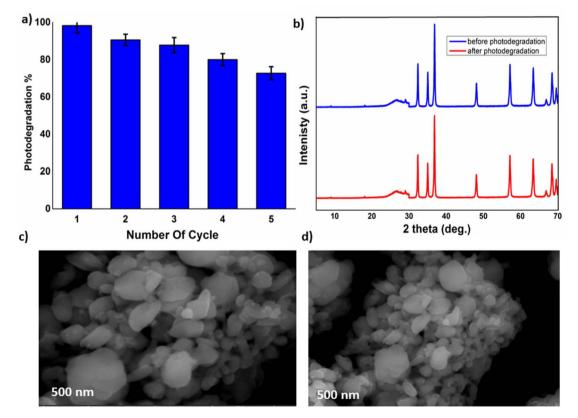
Fig. 13 (a) Reusability and recyclability study of the as-fabricated CdSQDs@ZnCr-LDO/ZnO on the photocatalytic efficiency in RhB photo-degradation. (b) XRD patterns of native and recycled catalyst after photodegradation process, (c and d) FE-SEM images of native and recycled catalyst, respectively.
