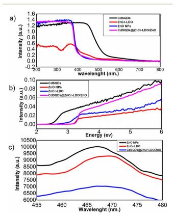
Fig. 8 (a) DRS spectra, (b) Tauc plots, and (c) PL spectra of the as-fabricated nanomaterials (ZnO NPs, ZnCr-LDO, CdSQDs@ZnCr-LDO/ZnO).
