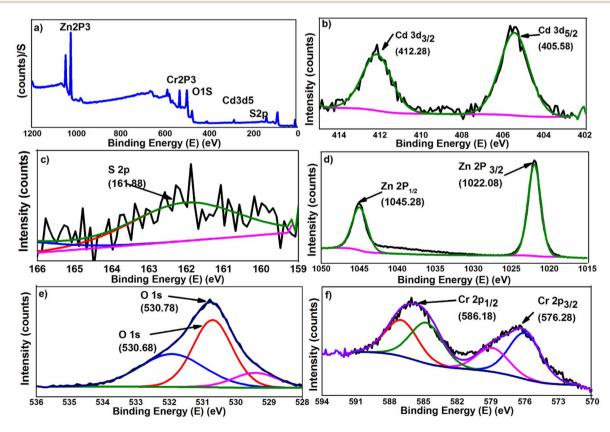
Fig. 6 (a) Sample survey XPS spectrum of CdSQDs@ZnCr-LDO/ZnO, High resolution XPS spectra of (b) Cd (3d), (c) S (2p), (d) Zn (2p), (e) O (1s), and (f) Cr (2p).
