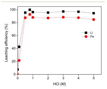
**Fig. 1** Effect of acid concentration on the leaching efficiency of Li and Fe from LFP material,  $S/L=20~g~L^{-1}$ , 2 hours, 500 rpm and room temperature. The invisible error bars indicate very small errors.
