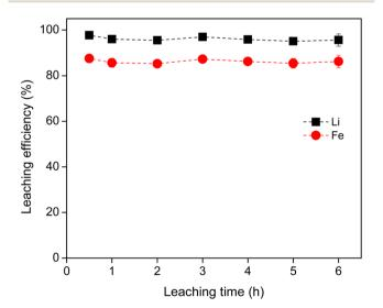
Fig. 3 Relationship between leaching time and leaching efficiency (%) of Li and Fe from LFP material, using 0.8 M HCl, with a S/L ratio of 10 and 40 g  $L^{-1}$ , at room temperature. The invisible error bars indicate very small errors.
