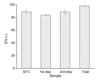
Fig. 7 Extraction percentage of Fe from the aqueous phase by  $[P_{44414}]$  Cl, using 90 wt% IL and a leachate with 4.5 M NaCl in a 3:2 aqueous: IL volume ratio, at 50 °C (the first column on the left) and at room temperature using two extraction steps (the remaining 3 columns).
