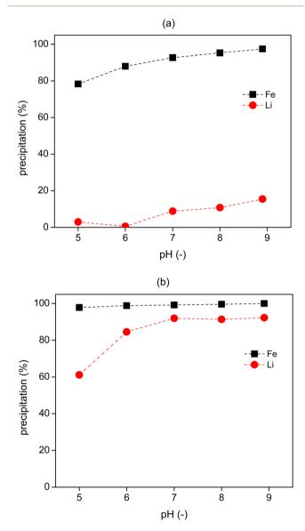
Fig. 9 Precipitation of lithium by addition of NaOH at room temperature and thereafter  $K_3PO_4$  solution at 60 °C to the raffinate obtained from the 2-stage cross-current solvent extraction process. (a) After adding NaOH to the raffinate, (b) after adding  $K_3PO_4$  solution.
