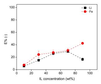
Fig. 4 Distribution ratio and extraction percentage of Li and Fe in  $[P_{44414}]Cl-HCl$  system, using 2.5 M HCl and varying wt% of IL, in a 3 : 2 aqueous: IL volume ratio, at 50 °C.
