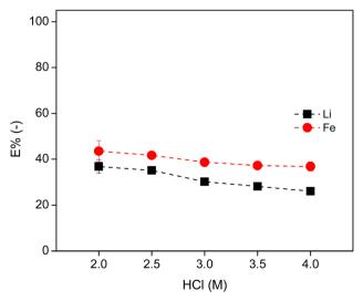
Fig. 5 Distribution ratio and E% of Li and Fe in the  $[P_{44414}]Cl-HCl$  system, using 90 wt% IL and varying HCl concentrations, in a 3:2 aqueous: IL volume ratio, at 50 °C. The invisible error bars indicate very small errors.
