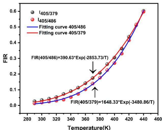
Fig. 10 Luminescence intensity ratio (FIR) of the LSGW:0.3Tb<sup>3+</sup> phosphor in the 290–440 K temperature range for FIR1 (405/379), and FIR2 (405/486).
