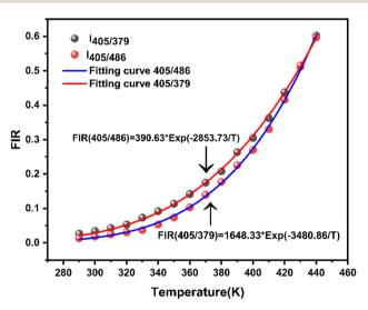
Fig. 10 Luminescence intensity ratio (FIR) of the LSGW:0.3Tb<sup>3+</sup>phosphor in the 290–440 K temperature range for FIR1 (405/379), and FIR2 (405/486).
