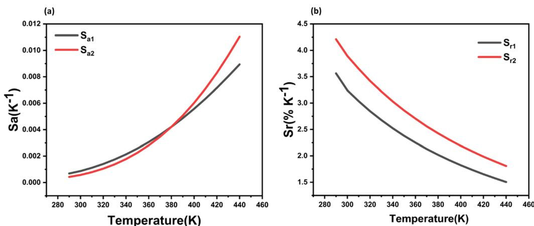
Fig. 11 (a) Absolute and, (b) relative thermal sensitivities obtained for the LSGW:0.3Tb<sup>3+</sup> phosphor in the 290–440 K temperature range.
