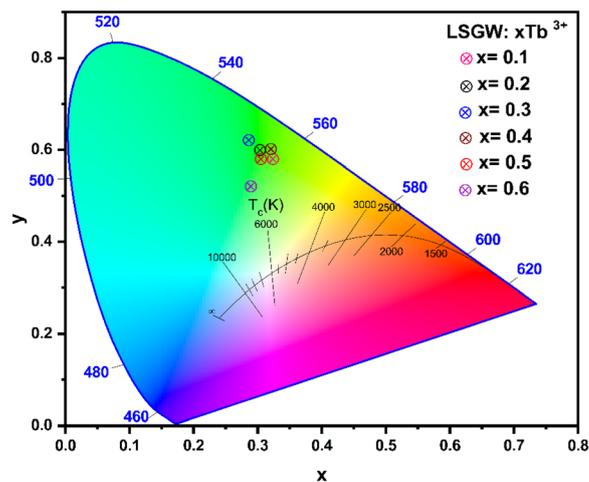
Fig. 8 CIE chromaticity diagram at different concentration of LSGW: $x\text{Tb}^{3+}$  ( $x = 0.1, 0.2, 0.3, 0.4, 0.5$  and  $0.6$ ) phosphor. As we use the same symbol, it cannot be seen the change of the CIE coordinates with the  $\text{Tb}$  concentration.
