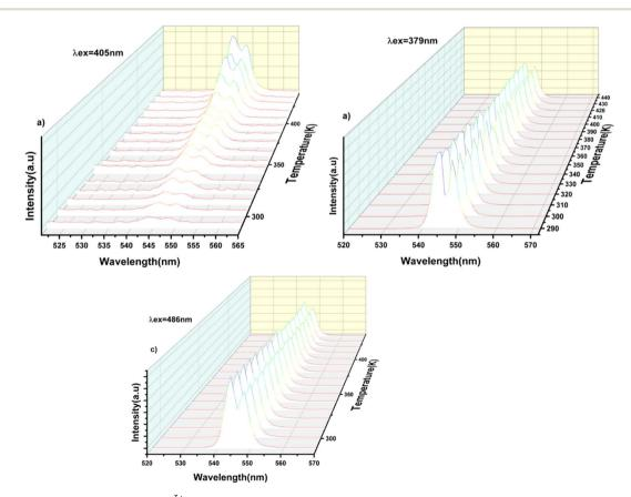
Fig. 9 Emission spectra of the LSGW:0.3Tb<sup>3+</sup> phosphor at different temperatures at: (a) 405 nm excitation (ESA), (b) 379 nm (GSA), (c) 486 nm (GSA).
