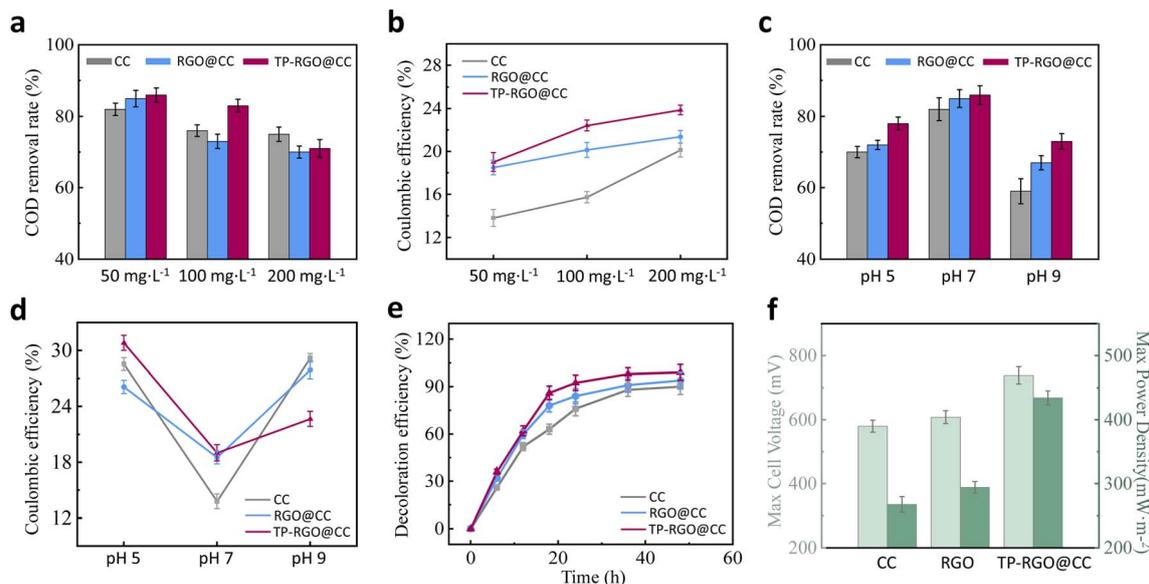
Fig. 4 (a) COD degradation rate of different anodes at different concentrations; (b) coulombic efficiency of different electrodes at different concentrations; (c) COD degradation rate of different anodes at different pH; (d) coulombic efficiency of different electrodes at different pH; (e) decolorization efficiency versus time at 50 mg L<sup>-1</sup>, pH 7; (f) the maximum power density and max cell voltage of MFCs is closely related to the amount of biomass.
