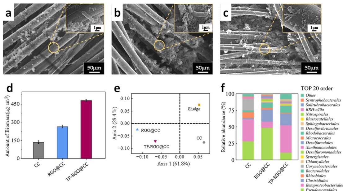
Fig. 5 SEM images of biofilm growth on (a) CC, (b) RGO@CC and (c) TP-RGO@CC anodes; (d) amount of biomass of anode; (e) principal coordinates analysis (PCoA); (f) the structure of microbial community at different anodes.
