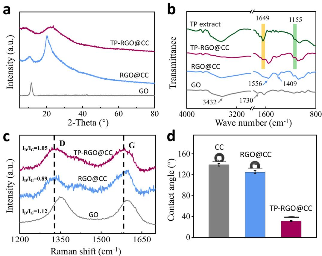
Fig. 2 (a) XRD spectra; (b) FTIR spectra; (c) Raman spectra and (d) contact angles of CC, RGO@CC, TP-RGO@CC anodes.
