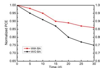
Fig. 7 Normalized PCE values of PSCs versus aging time (room temperature, RH: 35%, time: 30 days).
