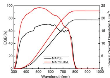
Fig. 6 EQE spectra and integrated current density of MAPbI<sub>3</sub> and MAPbI<sub>3</sub> + 1.0% BA.
