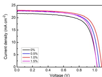
Fig. 4 *J*–*V* curves of PSCs based on 0, 0.5, 1.0, and 1.5% BA additive-MAPbI<sub>3</sub> films, respectively.
