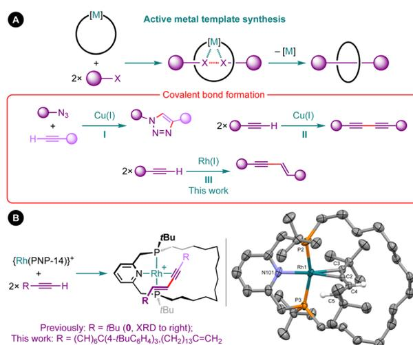
**Fig. 1** (A) Active metal template synthesis of interlocked molecules and (B) terminal alkyne dimerisation reactions promoted by macrocyclic rhodium(i) PNP pincer complexes. Solid-state structure of complex **0** shown with thermal ellipsoids drawn at 30% probability and most H-atoms omitted.
