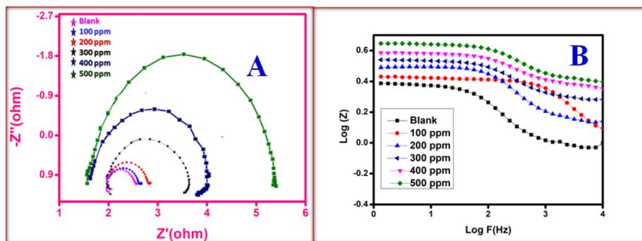
Fig. 6 Impedance plot for mild steel in 0.5 M blank and test solution (A) and (B) Bode plots.
