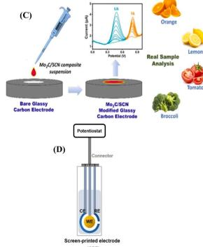
Fig. 4 GCEs modification processes for various vitamins detection. (A) Reproduced from ref. 60 with permission from Wiley-VCH, copyright 2024 and (B) reproduced from ref. 61 with permission from Wiley-VCH, copyright 2022 (C) reproduced from ref. 62 with permission from Elsevier, copyright 2023 (D) representation of SPE potentiostat adopted from ref. 64 permission under the terms of the CC-BY Creative Commons Attribution 4.0.
