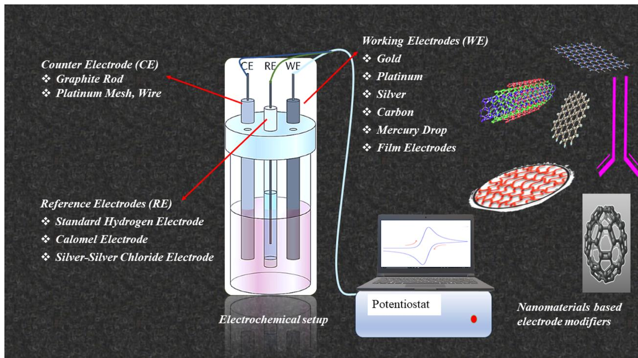
Fig. 3 Schematic representation of electrochemical setup and examples of respective electrode materials.
