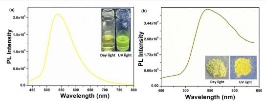
Fig. 4 Solution phase (a) and solid state (b) emission spectra of the compound H<sub>5</sub>L (inset is the photographs under daylight and UV light).
