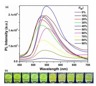
Fig. 5 Fluorescence emission spectra of (a)  $H_5L$  (excitation at 382 nm) in DMF/ $H_2O$  binary mixture. The percentage represents the volumetric fraction ( $f_W$ ) of  $H_2O$ , (b) optical images represent the AIEE of  $H_5L$  under UV light (excitation at 345 nm).
