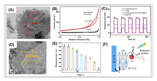
Fig. 7 (A) TEM image of A-CN. (B) Nitrogen adsorption—desorption isotherm curves for bulk CN and A-CN. (C) Photocurrent responses of bulk CN and A-CN. Adopted from ref. 163. Copyright 2020, with permission of Elsevier. (D) TEM images of PCN-S. (E) Photocurrent responses of the Au/PCN-S at various oxytetracycline concentrations. (F) The photocurrent generation mechanism of Au/PCN-S under visible light irradiation. Adopted from ref. 162. Copyright 2018, with permission of Elsevier.
