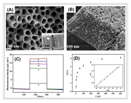
Fig. 4 SEM images of (A) TiO<sub>2</sub> NTs and (B) BiOI NFs/TiO<sub>2</sub> NTs. (C) Photocurrent responses of (a) TiO<sub>2</sub> NTs, (b) BiOI NFs/TiO<sub>2</sub> NTs, (c) aptamer/BiOI NFs/TiO<sub>2</sub> NTs, (d) BSA/aptamer/BiOI NFs/TiO<sub>2</sub> NTs, and (e) atrazine/BSA/aptamer/BiOI NFs/TiO<sub>2</sub> NTs. (D) Photocurrent change against atrazine concentrations. Adopted from ref. 67. Copyright 2021, with permission of Elsevier.
