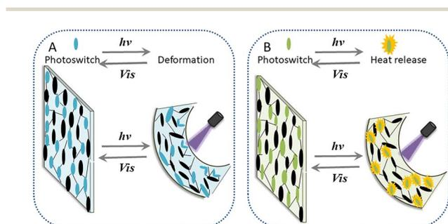
Fig. 1 (A) Opto-mechanical drive. (B) Photothermal drive.
