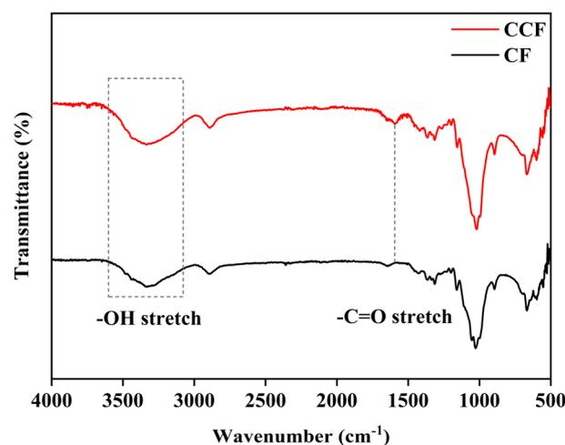
Fig. 1 FT-IR spectra of untreated CF and CCF.
