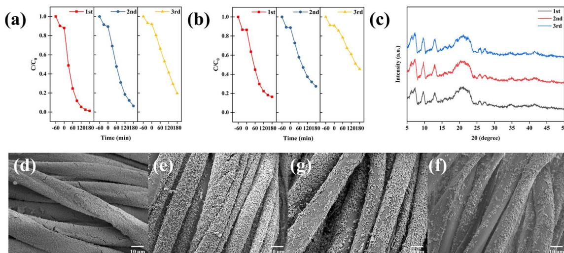
Fig. 12 Photocatalytic recycle degradation efficiency of RhB by using (a) CAU-17\_150@CCF and (b) CAU-17\_150; (c) XRD patterns of CAU-17\_150@CCF after each recycling application; SEM images of (d) initial CAU-17\_150@CCF, (e) 1st, (g) 2nd and (f) 3rd cycle.
