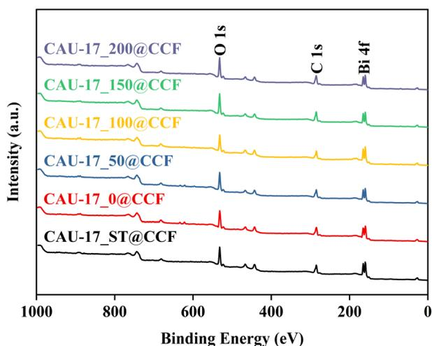
Fig. 6 XPS survey of CAU-17\_X@CCF and CAU-17\_ST@CCF.
