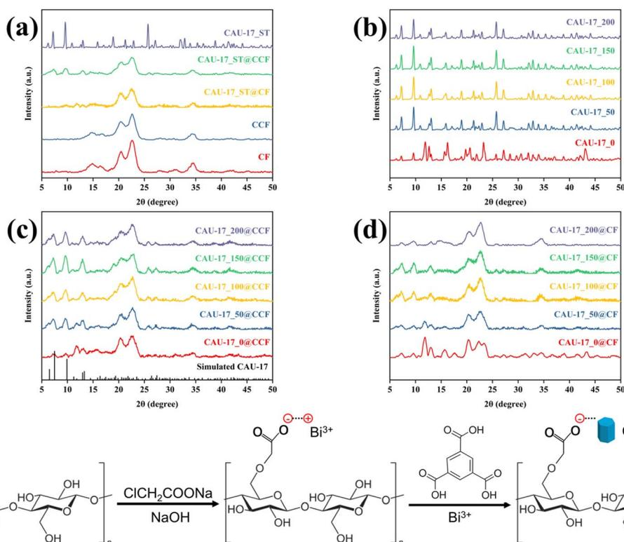
Fig. 3 XRD patterns of (a) MOF powder and cotton composite were obtained by the solvothermal route, CF, and bare CCF; (b) CAU-17\_X; (c) CAU-17\_X@CCF; (d) CAU-17\_X@CF; (e) schematic of the carboxymethylation and growth of CAU-17 on CCF.
