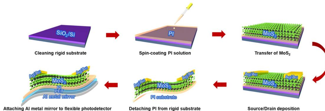
Fig. 1 Schematic fabrication process flow of the MoS<sub>2</sub>-based flexible photodetector on a PI substrate with a backside Al metal mirror.
