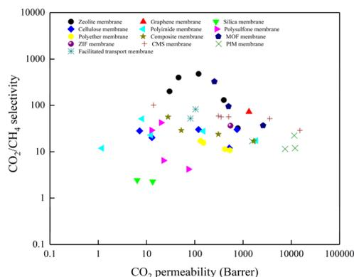
Fig. 9 CO<sub>2</sub>/CH<sub>4</sub> gas separation performance of different types of membranes.
