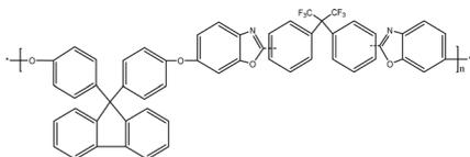
Fig. 7 Structure of the HPEI TR-polymer.<sup>116</sup>
