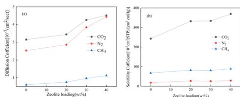
Fig. 4 (a) Diffusivity and (b) solubility of CO<sub>2</sub>, N<sub>2</sub>, and CH<sub>4</sub> in 6FDA-TrMPD/SAPO-34 MMMs with different zeolite loadings.<sup>89</sup>
