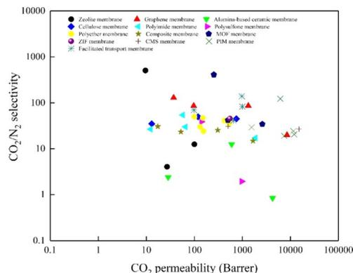
Fig. 10 CO<sub>2</sub>/N<sub>2</sub> gas separation performance of different types of membranes.
