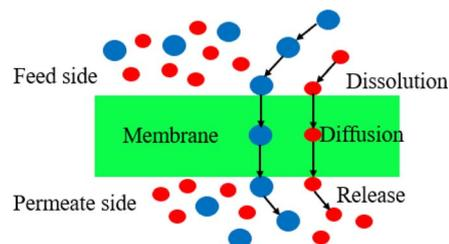
Fig. 2 Schematic diagram of solution permeation diffusion.
