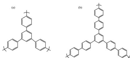
Fig. 8 Structure of (a) PPN1 and (b) PPN2.<sup>123</sup>
