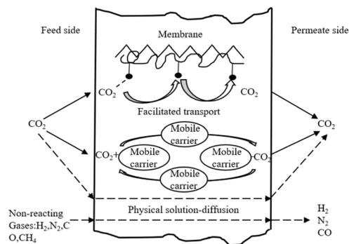
Fig. 3 Schematic diagram of the facilitated transport mechanism.<sup>10</sup>
