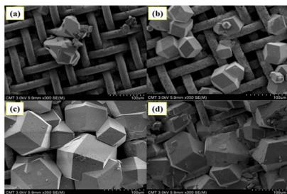
Fig. 6 FESEM images of ZIF-8 layers prepared on PDA-functionalized SSNs with different synthesis times: 8 h (a), 16 h (b), 24 h (c), and 48 h (d).<sup>110</sup>
