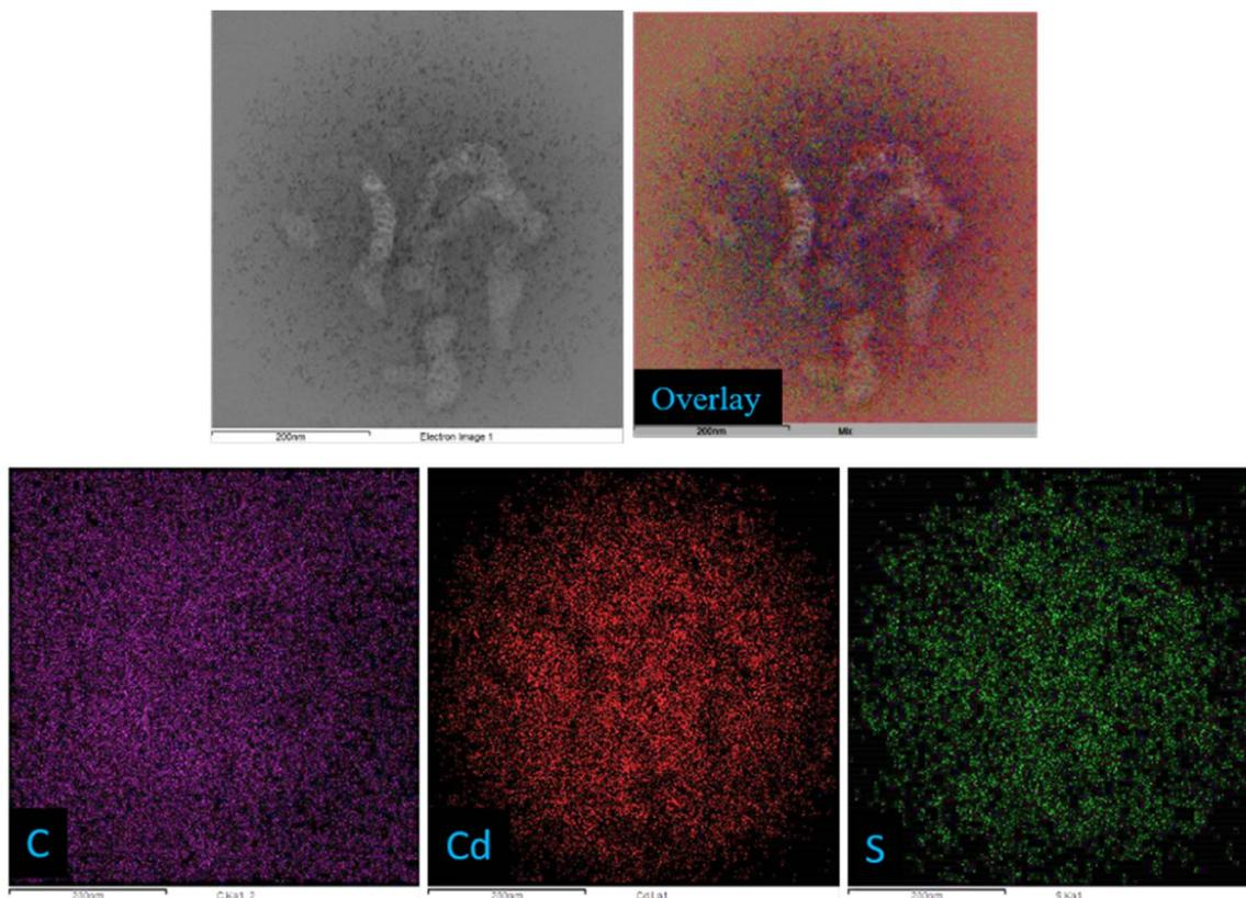
Fig. 3 Representative HAADF-STEM and the corresponding EDX mapping of elements C (violet), Cd (red), S (green) and the overlay of CD–CdS QD nanocomposite.
