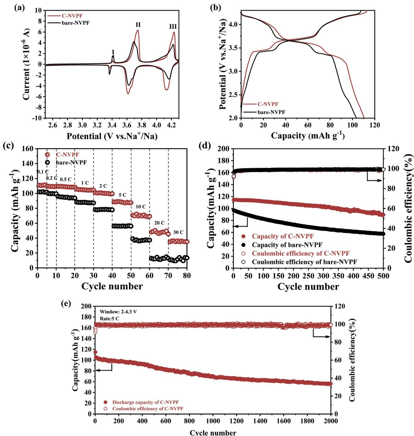
Fig. 5 (a) CV curves at a scan rate of 0.1  $\text{mV s}^{-1}$ , (b) typical charge-discharge curves, (c) rate properties, (d) cycling property at a 1C rate in a voltage range of 2.0–4.3 V, (e) cycling property at a 5C rate in a voltage range of 2.0–4.3 V of the bare-NVPF and C-NVPF electrodes.
