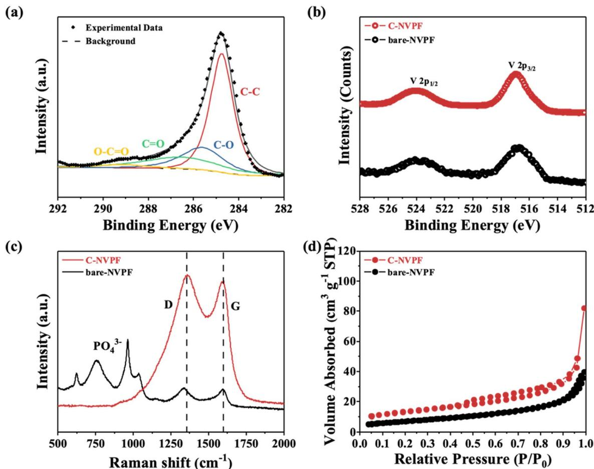
Fig. 4 (a) Electron energy spectrum of C (1s) for C-NVPF; (b) electron energy spectrum of V (2p); (c) Raman spectra; (d) N<sub>2</sub> adsorption and desorption curves for bare-NVPF and C-NVPF.
