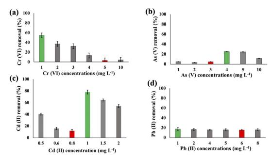
Fig. 2 Heavy metal (Cr(vi) (a), As(v) (b), Cd(ii) (c), and Pb(ii) (d)) removal efficiency of *A. variabilis* after 48 h at pH 8 with different initial concentrations. Error bars indicate standard deviation. Green and red bars indicate the maximum and minimum removal efficiency, respectively.
