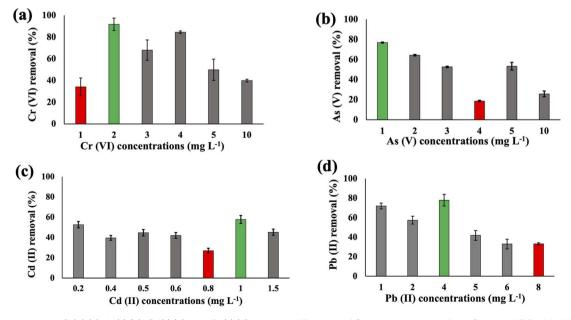
Fig. 1 The heavy metal Cr(vı) (a), As(v) (b), Cd(ıı) (c), and Pb(ıı) (d) removal efficiency of Synechocystis sp. after 48 h at pH 7.5 with different initial concentrations. Error bars indicate the standard deviation. Green and red bars indicate the maximum and minimum removal efficiency, respectively.
