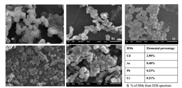
Fig. 9 SEM images of *Synechocystis* sp. before (a) and after Cd(II) (b), As(V) (c), Pb(II) (d), and Cr(VI) (e) adsorption. Quantitative analysis (f) of the HMs from EDS analysis.
