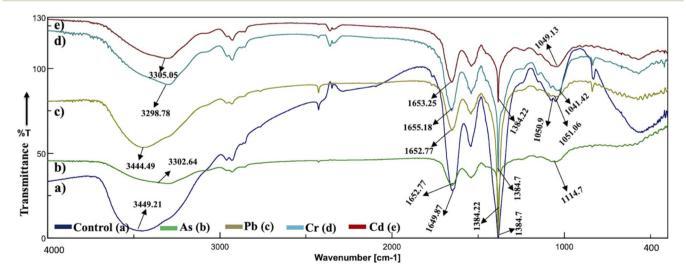
Fig. 6 Active center analysis by FT-IR spectrum of Synechocystis sp. before (control – (a)) and after  $(As(v) - (b), Pb(u) - (c), Cr(v_l) - (d), and Cd(u) - (b), Pb(u) - (c), Cr(v_l) - (d), and Cd(u) - (b), Pb(u) - (b), Pb(u) - (c), Cr(v_l) - (d), and Cd(u) - (b), Pb(u) - (b), Pb(u) - (c), Cr(v_l) - (d), and Cd(u) - (d), and C$ (e)) HM adsorption.
