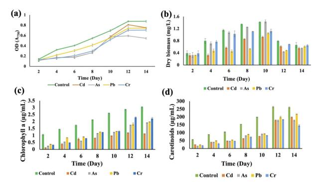
Fig. 3 Effects of HMs on optical density (OD<sub>730</sub>) (a), dry biomass (b), chlorophyll a (c), and carotenoid (d) production of *A. variabilis* under HM (1 mg L<sup>-1</sup> Cd( $_{\rm II}$ ), 4 mg L<sup>-1</sup> As( $_{\rm V}$ ), 1 mg L<sup>-1</sup> Pb( $_{\rm II}$ ), and 1 mg L<sup>-1</sup> Cr( $_{\rm V}$ )) stress during the cultivation time. Error bars indicate standard deviation.
