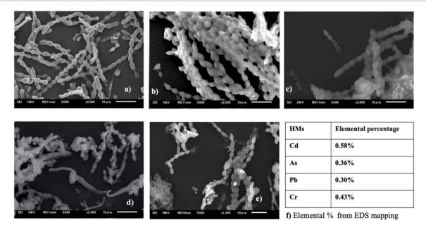
Fig. 8 SEM images of A. variabilis before (a) and after Cd( $\shortparallel$ ) (b), As( $\lor$ ) (c), Pb( $\shortparallel$ ) (d), and Cr( $\lor$ ) (e) adsorption. Quantitative analysis (f) of HMs from EDS analysis.
