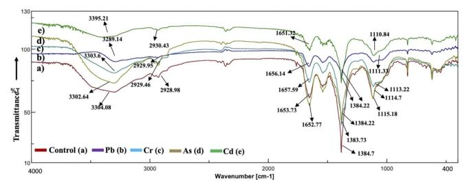
Fig. 7 Active center analysis by FT-IR spectrum of A. variabilis before (Control – (a)) and after (Pb( $_{\parallel}$ ) – (b), Cr( $_{\parallel}$ ) – (c), As( $_{\parallel}$ ) – (d), and Cd( $_{\parallel}$ ) – (e))
