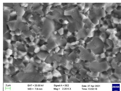
Fig. 10 Fracture cross sections of alpha alumina.
