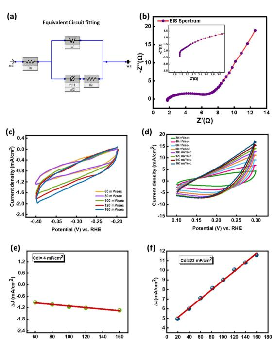
Fig. 7 (a) Equivalent circuit diagram. (b) Nyquist plot of NiCo-MOF with zoomed-in image in the inset. (c) Cyclic voltammograms of NiCo-MOF for HER. (d) CV scans for OER. (e)  $C_{\rm cl}$  value of required sample in case of hydrogen evolution. (f)  $C_{\rm cl}$  graph of oxygen evolution of the catalyst.
