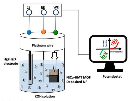
Fig. 5 Three-electrodes setup for catalysis of water.
