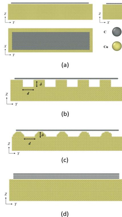
Fig. 1 APG–Cu interfacial thermal resistance model (a) monolayer APG model (b) cylindrical surface of copper (c) rectangular surface of copper (d) multilayer APG–Cu interfacial thermal resistance model.
