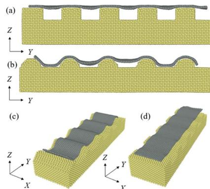
Fig. 7 Different surface micromorphology of APG–Cu interface at the end of simulation with a depth of  $\delta = 1.25$  nm (a) rectangular surface front view; (b) cylindrical surface front view; (c) cylindrical surface top view; (d) rectangular surface top view.
