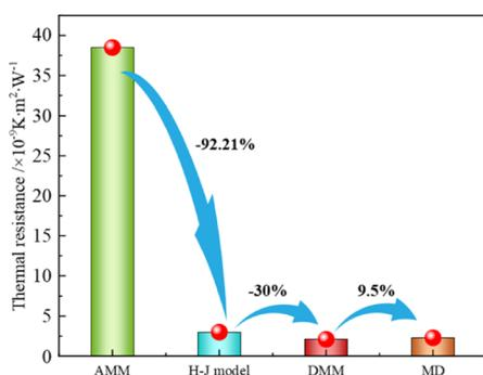
Fig. 11 Comparison of interfacial thermal resistance between our calculation result and published results.<sup>29–31</sup>
