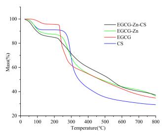
Fig. 3 Thermogravimetric analysis of the samples.
