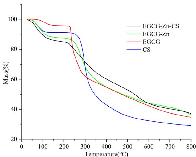
Fig. 3 Thermogravimetric analysis of the samples.
