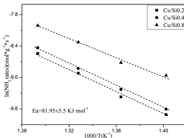
Fig. 11 The kinetic results of  $\text{NH}_3$  oxidation over the Cu/SAPO-34 catalysts. The inlets consisted of 500 ppm  $\text{NH}_3$  and 5%  $\text{O}_2$ , with  $\text{N}_2$  as the balance. The kinetic steady-state tests were conducted from  $440\text{ }^\circ\text{C}$  to  $500\text{ }^\circ\text{C}$ .
