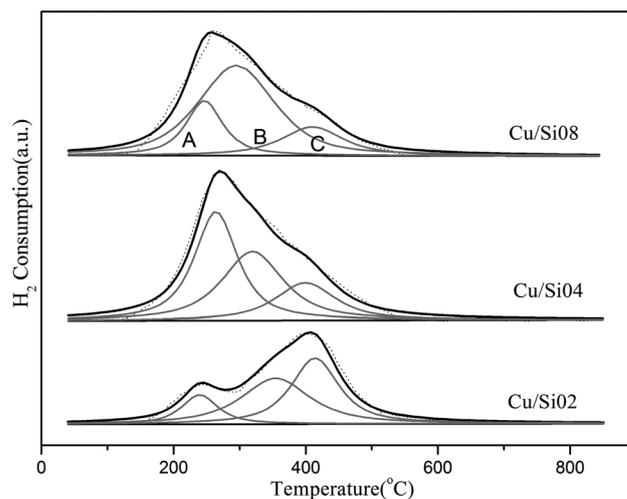
Fig. 7 The H<sub>2</sub>-TPR results for Cu/SAPO-34. Dashed line represents the fitting results.
