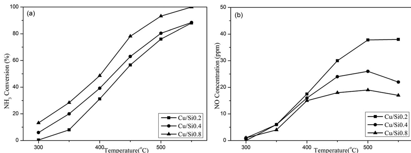
Fig. 9 The NH<sub>3</sub> oxidation activity over Cu/SAPO-34 catalysts. (a) NH<sub>3</sub> conversion; (b) NO generation. The inlets consisted of 500 ppm NH<sub>3</sub> and 5% O<sub>2</sub>, with N<sub>2</sub> as the balance. The volume hourly space velocity in the experiments was kept at 30 000 h<sup>-1</sup>.
