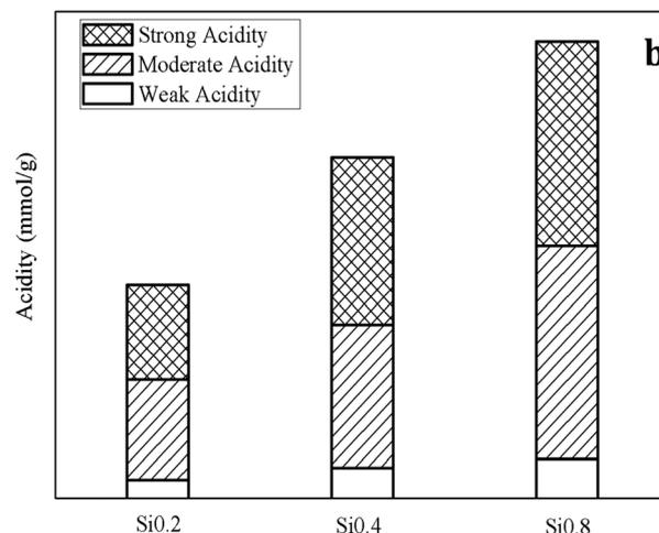
Fig. 3 The NH<sub>3</sub>-TPD profiles and the acid contents for the SAPO-34 supports.
