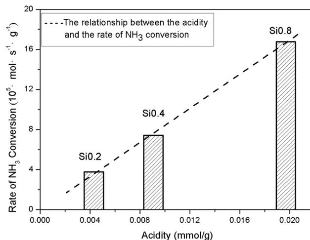
Fig. 6 The relationship between the acidity and the NH<sub>3</sub> conversion rate at 300 °C.
