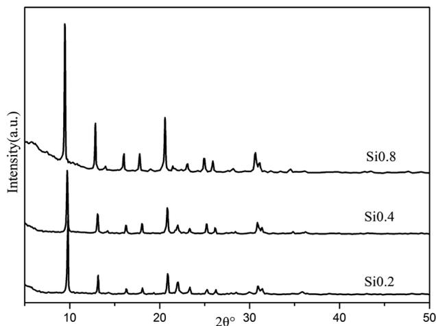
Fig. 1 The XRD profiles of the SAPO-34 supports.
