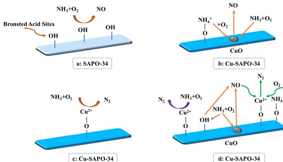
Scheme 1 The NH<sub>3</sub> oxidation mechanism of the SAPO-34 support and Cu/SAPO-34 catalyst.
