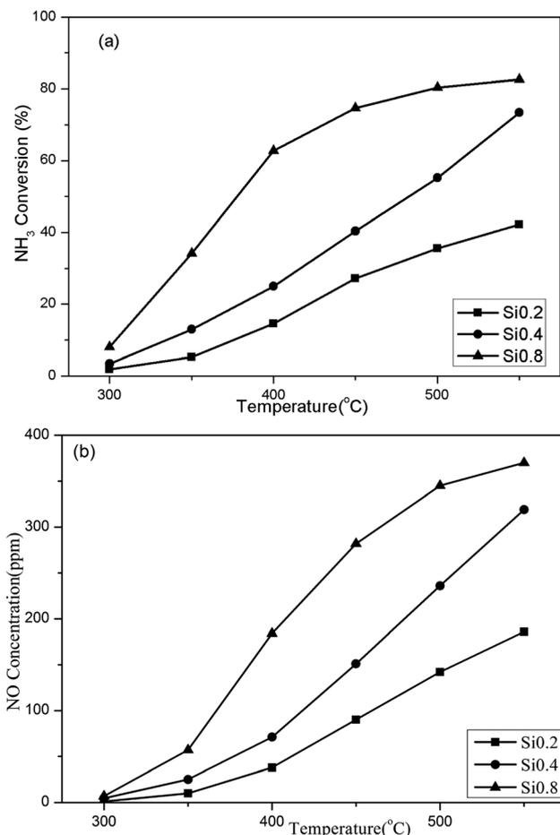
Fig. 4 NH<sub>3</sub> oxidation activities over the SAPO-34 supports. (a) The NH<sub>3</sub> conversion; (b) the NO conversion. The inlets consisted of 500 ppm NH<sub>3</sub> and 5% O<sub>2</sub>, with N<sub>2</sub> as the balance. The volume hourly space velocity in the experiments was kept at 30 000 h<sup>-1</sup>.
