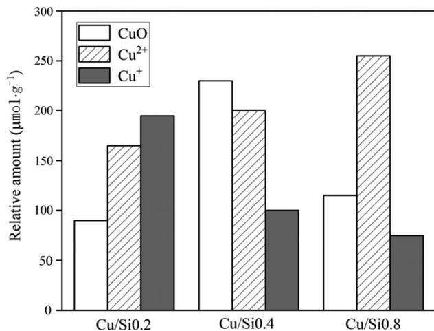
Fig. 8 The relative amount of CuO, isolated Cu<sup>2+</sup> ions and Cu<sup>+</sup> on three catalysts quantified by the H<sub>2</sub>-TPR profile.
