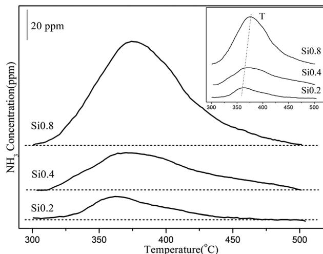
Fig. 5 The NH<sub>3</sub>-TPD profiles of the SAPO-34 supports at 300 °C.
