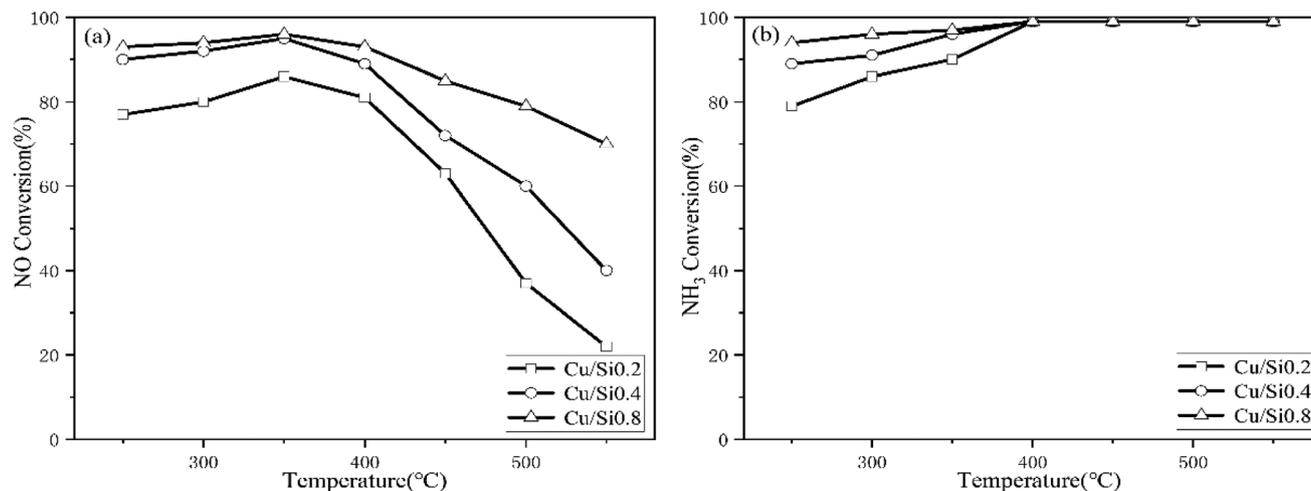
Fig. 10 The  $\text{NH}_3$  SCR activity over Cu/SAPO-34 catalysts. (a) NO conversion; (b)  $\text{NH}_3$  conversion. The inlets consisted of 500 ppm NO, 500 ppm  $\text{NH}_3$  and 5%  $\text{O}_2$ , with  $\text{N}_2$  as the balance. The volume hourly space velocity in the experiments was kept at  $30\,000\text{ h}^{-1}$ .
