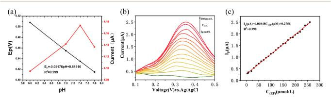
Fig. 3 (a) The plots of pH with response current and response potential in 0.1 M PBS containing 100  $\mu$ M EP. (b) DPV of  $K_2Fe_4O_7/GCE$  for different EP concentrations in 0.1 M PBS (pH = 7.4). (c) Plots of the response current and EP concentrations (2-260  $\mu$ M).
