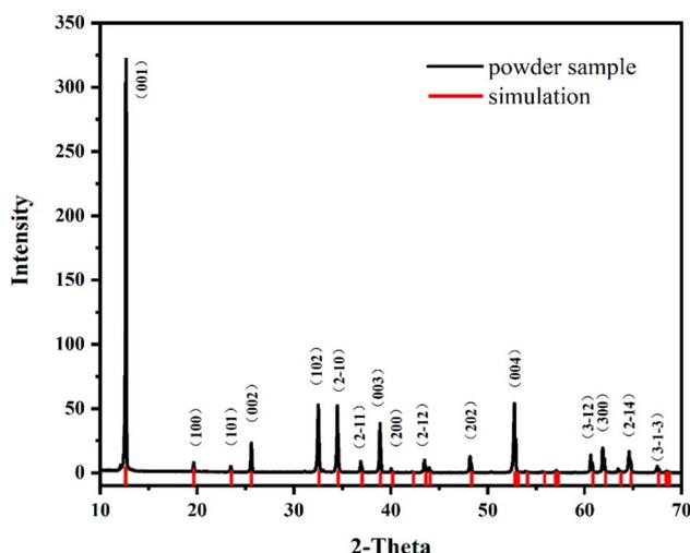
Fig. 1 The simulation and powder XRD patterns of K<sub>2</sub>Fe<sub>4</sub>O<sub>7</sub>.
