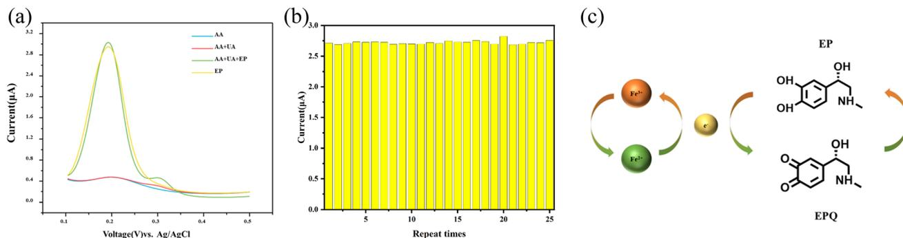
Fig. 4 (a) DPV response of  $K_2Fe_4O_7$ /GCE in 0.1 M PBS (pH = 7.4) containing 1 mM AA; 1 mM AA and 100  $\mu$ M UA; 100  $\mu$ M UA and 100  $\mu$ M EP; 100  $\mu$ M EP respectively. (b) Results of eight independent tests of  $K_2Fe_4O_7$ /GCE. (c) Brief detection mechanism.
