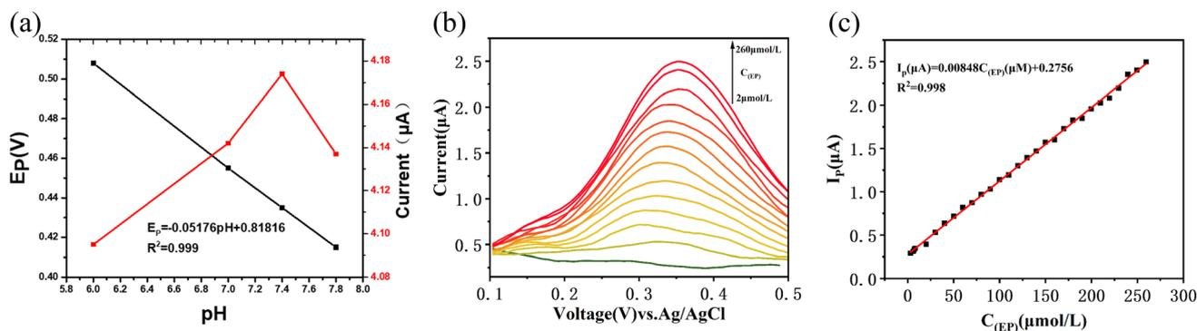
Fig. 3 (a) The plots of pH with response current and response potential in  $0.1\text{ M}$  PBS containing  $100\text{ }\mu\text{M}$  EP. (b) DPV of  $K_2Fe_4O_7$ /GCE for different EP concentrations in  $0.1\text{ M}$  PBS ( $\text{pH} = 7.4$ ). (c) Plots of the response current and EP concentrations ( $2\text{--}260\text{ }\mu\text{M}$ ).
