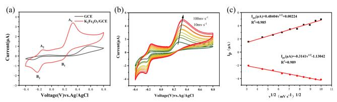
Fig. 2 (a) CV of bare GCE and  $K_2Fe_4O_7/GCE$  in 0.1 M PBS (pH = 7.4) containing 100  $\mu$ M EP. (b) CVs of  $K_2Fe_4O_7/GCE$  in 0.1 M PBS (pH = 7.4) containing 100 µM EP at scan rates of 10–100 mV s<sup>-1</sup>. (c) The plots of response currents and the square root of scan rate.
