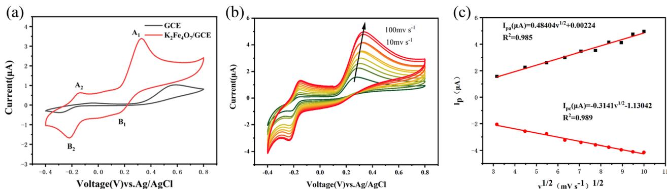
Fig. 2 (a) CV of bare GCE and K<sub>2</sub>Fe<sub>4</sub>O<sub>7</sub>/GCE in 0.1 M PBS (pH = 7.4) containing 100  $\mu\text{M}$  EP. (b) CVs of K<sub>2</sub>Fe<sub>4</sub>O<sub>7</sub>/GCE in 0.1 M PBS (pH = 7.4) containing 100  $\mu\text{M}$  EP at scan rates of 10–100  $\text{mV s}^{-1}$ . (c) The plots of response currents and the square root of scan rate.
