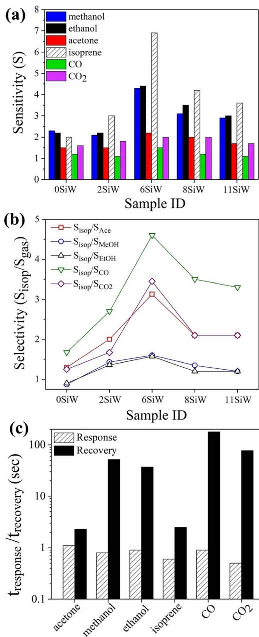
Fig. 5 (a) Comparison of gas sensitivities measured at 350 °C for isoprene, methanol, ethanol, acetone, CO and CO<sub>2</sub> with films containing different amounts of Si. (b) Isoprene selectivity over other gases. (c) Response and recovery times of the above gases measured with 6SiW at 350 °C.
