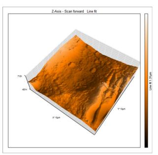
AFM for Al after immersion 0.5 M NaOH in the absence (a) and presence (b) of 0.0112 M of isoprinosine inhibitor.
