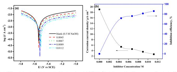
Fig. 3 (a) Potentiodynamic polarization graphs of aluminum electrode in 0.50 M NaOH solution containing different amounts of isoprinosine. (b) The effect of increasing concentration of isoprinosine on the current density and the inhibition efficiency.
