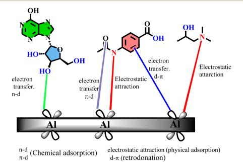
Fig. 10 Mechanism of adsorption of isoprinosine on aluminum surface.
