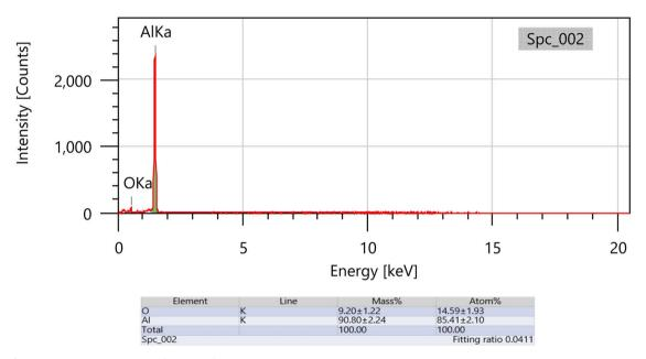
SEM/EDX for Al after immersion 0.5 M NaOH in the absence of isoprinosine.
