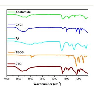
Fig. 2 FT-IR spectra of four components and ETG-acetamide.
