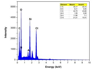
Fig. 6 Energy-dispersive X-ray spectroscopy for ETG-acetamide.
