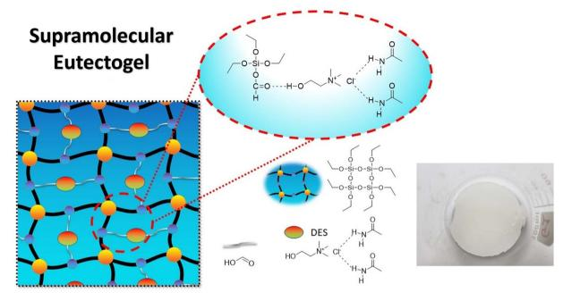
Fig. 1 The structure of ETG-acetamide.
