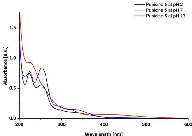
Fig. 3 UV-Vis spectrum of C<sub>11</sub>-punicine **5**.
