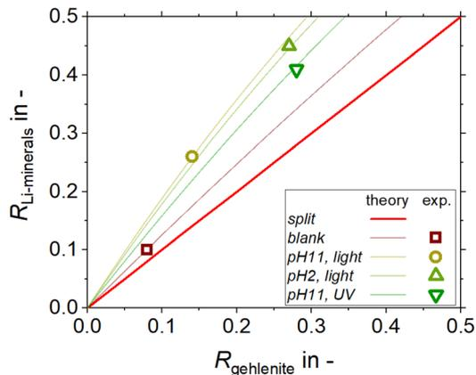
Fig. 12 Fuerstenau upgrading diagram for the mixed mineral micro flotation tests with 2.00 g of a 1 : 1 mixture of  $\text{LiAlO}_2$  and gehlenite,  $1 \times 10^{-5} \text{ M } C_{11}$ -punicine 5 ( $C_{11}$ ),  $1.2 \times 10^{-3} \text{ g l}^{-1}$  pine oil, conditioning time 3 min, flotation for 3 min with  $32 \text{ cm}^3 \text{ min}^{-1}$  air flow and 250 ml of distilled water.
