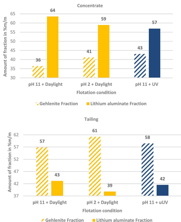
Fig. 11 The mass fraction % of lithium aluminate and gehlenite present in the concentrate and the tailing of their mixed micro flotation obtained from quantitative XRD measurements.
