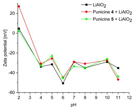
Fig. 14 Zeta potential of pure lithium aluminate, lithium aluminate with  $2.4 \mu\text{l}$  of  $42.5 \text{ mmol l}^{-1}$  punicine 4 and lithium aluminate with  $2.4 \mu\text{l}$  of  $42.5 \text{ mmol l}^{-1}$  punicine 5 in distilled water and under different pH values.
