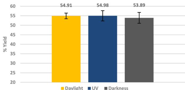
Fig. 7 Flotation of lithium aluminate using sodium oleate 1% wt as a collector. The conditioning was as following: 60  $\mu\text{l}$  collector ( $1 \times 10^{-5}$  M), 1 min mixing, 30  $\mu\text{l}$  frother, 1 min mixing, stirring speed 500 rpm, air flow rate 32 ml min<sup>-1</sup> using 250 ml distilled water and flotation time 3 min.
