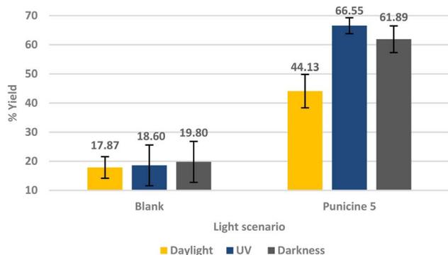
Fig. 6 Flotation of lithium aluminate using C<sub>11</sub>-punicine 5 as a collector under irradiation in daylight (yellow), in the dark (black), and under UV-light (blue). The conditioning was as following: 120  $\mu\text{l}$  collector ( $2 \times 10^{-5}$  M), 1 min mixing, 30  $\mu\text{l}$  frother, 1 min mixing, stirring speed 500 rpm, air flow rate 32 ml min<sup>-1</sup> using 250 ml distilled water and flotation time 3 min at pH 11.
