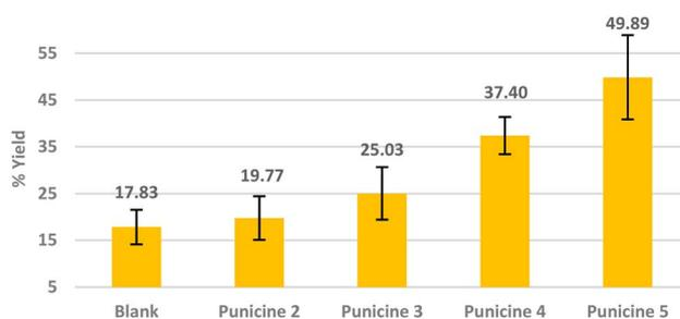
Fig. 5 Comparison of the recovery rates in the presence of the collectors 2–5 under identical conditions, i.e. 2.00 g of  $\text{LiAlO}_2$ , 1 min of mixing (500 rpm) with 25 ml of distilled water, 60  $\mu\text{l}$  ( $1 \times 10^{-5}$  M) of the corresponding collector, 1 min of mixing, 30  $\mu\text{l}$  of frother, and another 1 min of mixing. The flotation was done for 3 min at an air flow rate  $32 \text{ ml min}^{-1}$  using 250 ml distilled water in daylight at pH 11.
