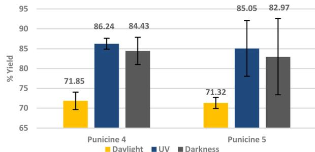
Fig. 9 Flotation of lithium aluminate using punicines 4 and 5 as collector at pH 11, and under different lighting conditions. The conditioning was as follows: 600  $\mu\text{l}$  collector ( $1 \times 10^{-4}$  M), 1 min mixing, 30  $\mu\text{l}$  frother, 1 min mixing, stirring speed 500 rpm, air flow rate 32  $\text{ml min}^{-1}$  using 250 ml distilled water and flotation time 5 min.
