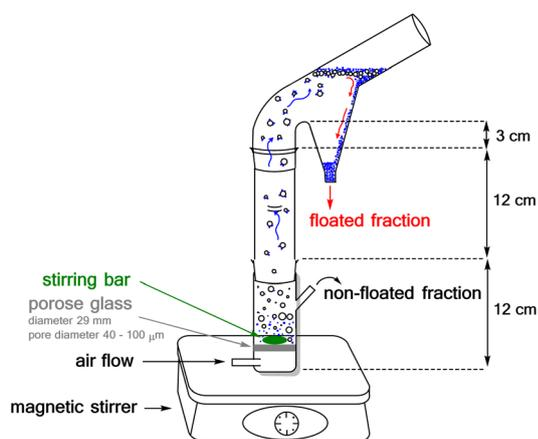
Fig. 15 Pictorial representation of the Hallimond tube used.
