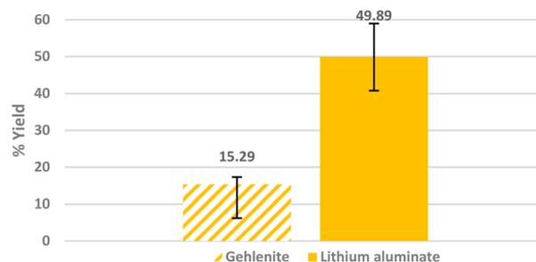
Fig. 10 Single mineral flotation of lithium aluminate and gehlenite using  $C_{11}$ -punicine 5 as collector at pH 11 for lithium aluminate and pH 5.8 for gehlenite in daylight. The conditioning was as follows: 60  $\mu\text{l}$  collector, 1 min mixing, 30  $\mu\text{l}$  frother, 1 min mixing, stirring speed 500 rpm, air flow rate 32  $\text{cm}^3 \text{min}^{-1}$  using 250 ml distilled water and flotation time 3 min.
