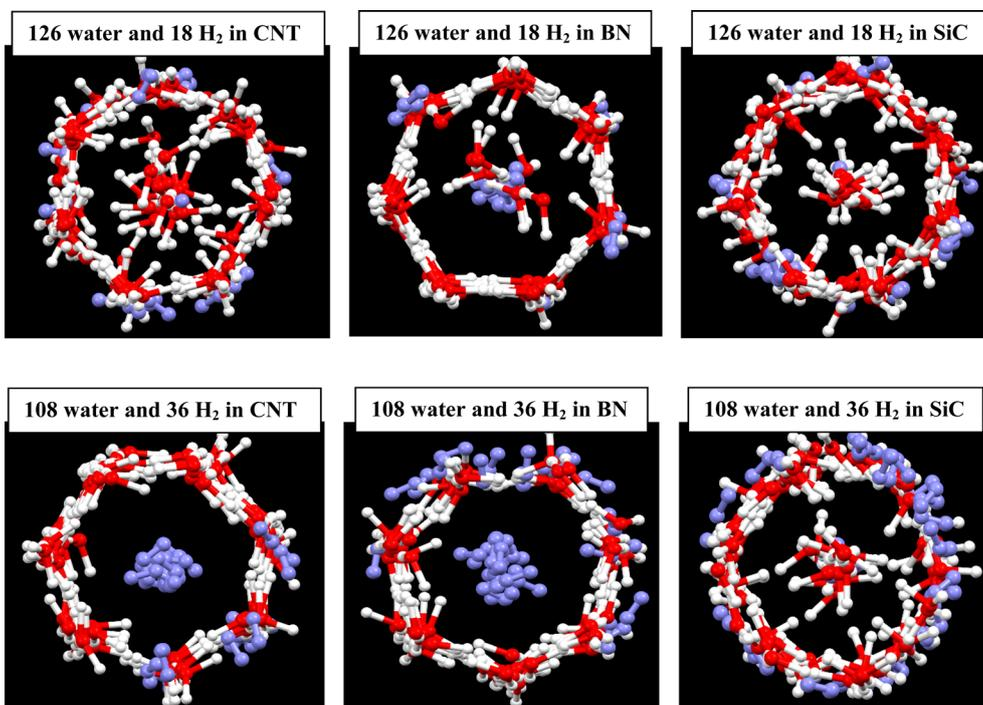
Fig. 2 H<sub>2</sub> clathrate formed in the different nanotubes. The oxygen atoms are shown in red color, hydrogen atoms in white, and hydrogen molecules in violet.
