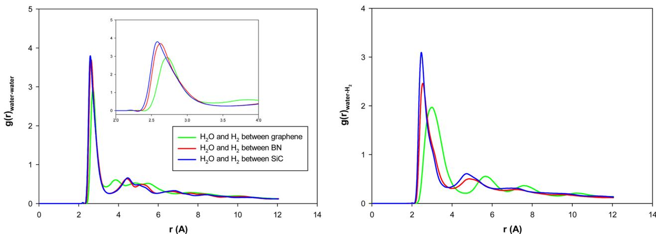
Fig. 5 Water-water and water-gas RDFs for the different surface systems.
