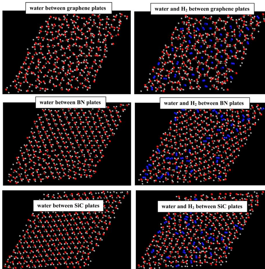
Fig. 4 Ice and H<sub>2</sub> clathrate structures formed between different surface systems. The oxygen atoms are shown in red color, hydrogen atoms in white, and H<sub>2</sub> molecules in blue.
