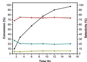
Fig. 2 Time-dependent performance profile of 1%Ru(Cl)/ZrO<sub>2</sub>(400) catalyst. Reaction conditions: 2 mmol styrene, styrene/Ru = 83, 0.1 g *n*-decane, 5 mL methanol, *P* = 0.5 MPa, *T* = 160 °C. (■) Conversion of styrene, (▲) selectivity of L, (▼) selectivity of B, (●) selectivity of others.
