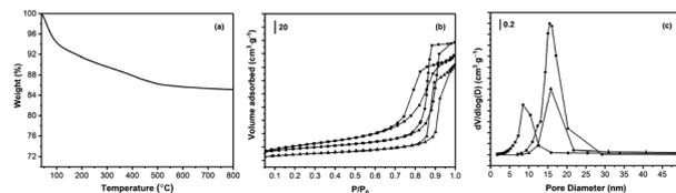
Fig. 1 (a) TG curve of dried  $\text{ZrO}_2$ ; (b)  $\text{N}_2$  adsorption–desorption isotherms of calcined  $\text{ZrO}_2$ ; and (c) BJH pore size distribution of calcined  $\text{ZrO}_2$ . (■)  $\text{ZrO}_2(400)$ , (●)  $\text{ZrO}_2(500)$ , (▲)  $\text{ZrO}_2(600)$ .
