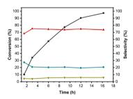
Fig. 2 Time-dependent performance profile of  $1\%Ru(Cl)/ZrO_2(400)$  catalyst. Reaction conditions: 2 mmol styrene, styrene/Ru = 83, 0.1 g n-decane, 5 mL methanol, P = 0.5 MPa, T = 160 °C. ( $\blacksquare$ ) Conversion of styrene, ( $\blacktriangle$ ) selectivity of L, ( $\blacktriangledown$ ) selectivity of B, ( $\bullet$ ) selectivity of others.
