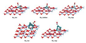
Fig. 6 The optimized geometries of CO adsorption on Ru<sub>3</sub>/m- $ZrO_2(-111)_{V\ddot{o}}$  and  $Ru_7/m-ZrO_2(-111)_{V\ddot{o}}$
