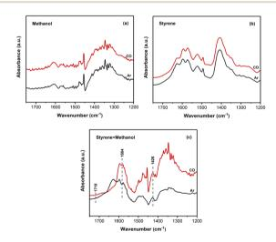
Fig. 5 In situ FTIR spectra of (a) methanol adsorption, (b) styrene adsorption, and (c) the hydroesterification of styrene over 1%Ru(CI)/ ZrO<sub>2</sub>(400) at 160 °C under Ar and CO.
