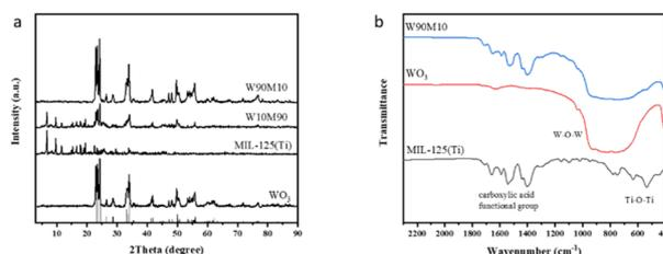
Fig. 1 (a) The XRD patterns and (b) the FTIR spectra of WO<sub>3</sub>, MIL-125 (Ti) and W<sub>x</sub>M<sub>y</sub>.
