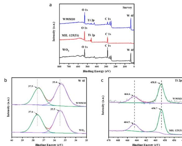
Fig. 3 (a) XPS survey spectra of  $\text{WO}_3$ , MIL-125 (Ti) and  $\text{W}_x\text{M}_y$ , (b) HR-XPS spectra of W 4f for  $\text{WO}_3$ ,  $\text{W}_x\text{M}_y$ , (c) HR-XPS spectra of Ti 2p for MIL-125 (Ti),  $\text{W}_x\text{M}_y$ .
