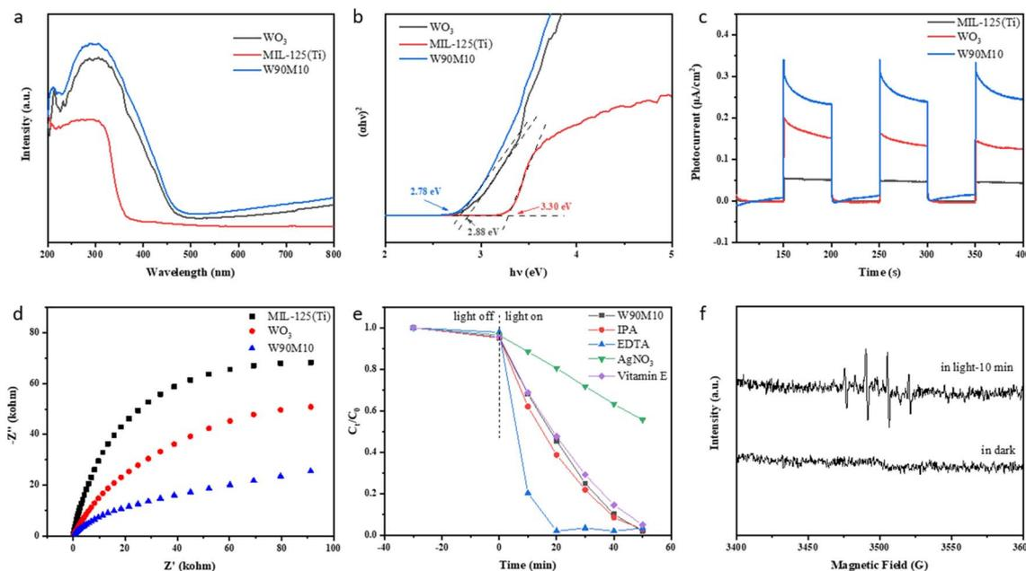
Fig. 5 (a) UV-vis DRS and (b)  $E_g$  plots; (c) photocurrent responses and (d) EIS Nyquist plots of  $\text{WO}_3$ , MIL-125 (Ti) and W90M10; (e) free radical capture experiment for Cr(vi) reduction, (f) DMPO spin-trapping ESR technology for detection of  $\cdot\text{OH}$ .
