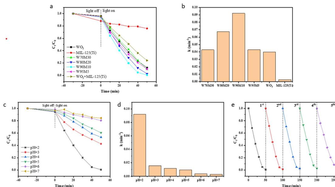
Fig. 4 (a) Photocatalytic reduction efficiency and (b) rate constant  $k$  of Cr(VI) with different composite ratios of catalysts; (c) photocatalytic reduction efficiency and (d) rate constant  $k$  of Cr(VI) at different pH; (e) cyclic test of Cr(VI) reduction by W90M10 under visible light catalysis.
