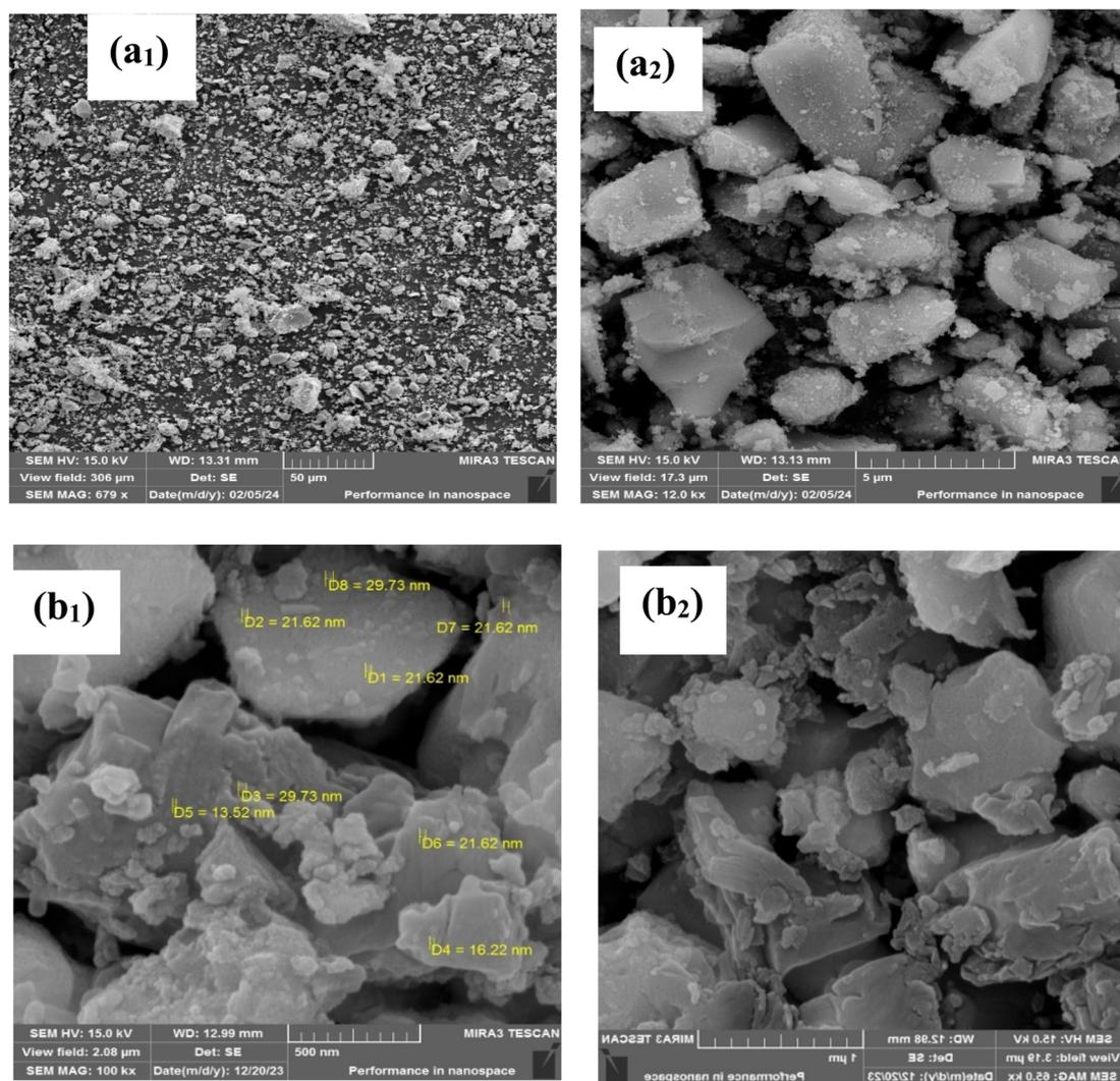
Fig. 3 FESEM images of (a<sub>1</sub> and a<sub>2</sub>) LDH@PTRMS and (b<sub>1</sub> and b<sub>2</sub>) LDH@PTRMS@DCMBA@CuI catalyst.
