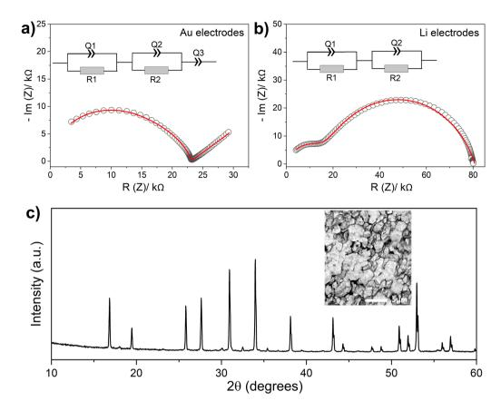
Fig. 5 (a) The impedance plot of hot-pressed 0.3Ga-doped LLSO collected at 40 °C using gold electrodes, and fitted using the [R1Q1][R2Q2][Q3] eguivalent circuit (the inset). (b) The impedance plot of hot-pressed 0.3Ga-doped LLSO collected at 40 °C using lithium electrodes, and fitted using the [R1Q1][R2Q2] equivalent circuit (the inset). (c) XRD pattern and SEM image (the inset) of hot-pressed 0.3Ga-doped LLSO.
